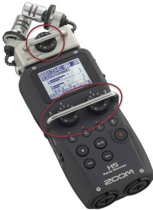
Figure 4-10. The gain knobs on the Zoom H5 portable recorder
