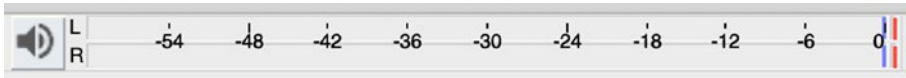
Figure 8-24. The Audacity meter is telling you that the audio has peaked at some point
