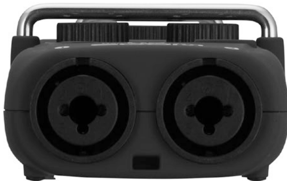
Figure 6-18. If using a Zoom H5, plug the TRS connector into these inputs (photo courtesy of Zoom)
