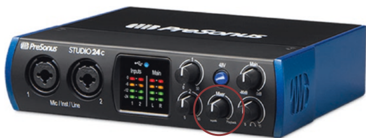
Figure 7-26. The knob to control direct monitoring on the Presonus Studio 24c
