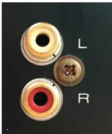
Figure 6-19. An RCA output
