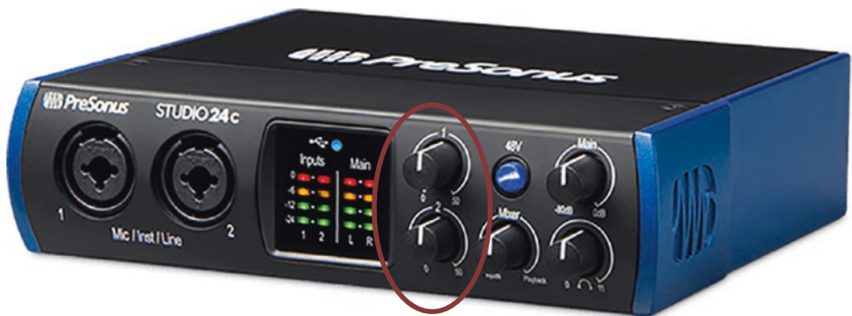
Figure 4-9. The two gain knobs on the PreSonus Studio 24c audio interface
