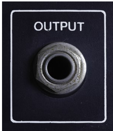
Figure 6-15. A quarter inch output socket (Simon Ashton/Shutterstock.com)
