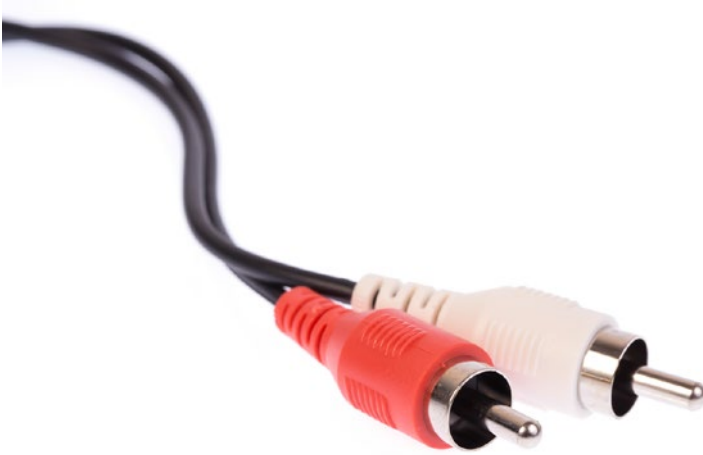
Figure 6-20. An RCA connector (Yellow Cat/Shutterstock.com)
