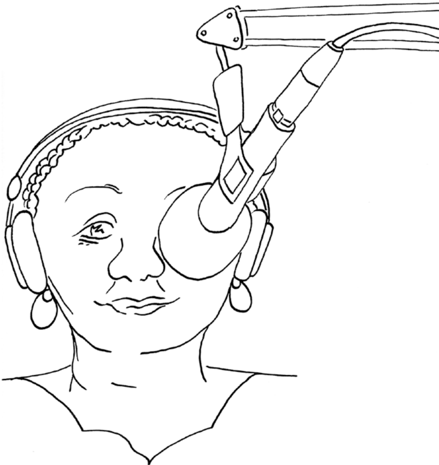
Figure 4-7. When recording a voice-over, position the microphone above the level of the speaker's mouth pointing down
