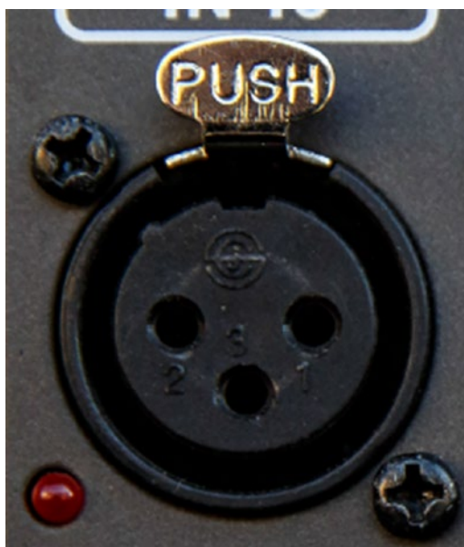
Figure 6-4. An XLR input (Piotr Piatrouski/Shutterstock.com)
