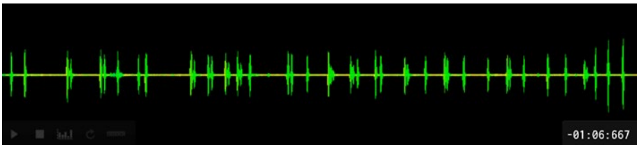
Figure 9-4. An audio clip from freesound.org that looks to have been recorded at a healthy level
