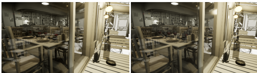
(a) Ray traced translucency with two refraction events: 16.2 ms (b) Half-resolution hybrid translucency with only the top layer traced: 4 ms + 1.5 ms
