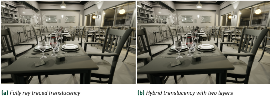
Figure 50-4. Hybrid translucency replicates the most important visual enhancements of full ray tracing while continuing to support rasterized elements.
