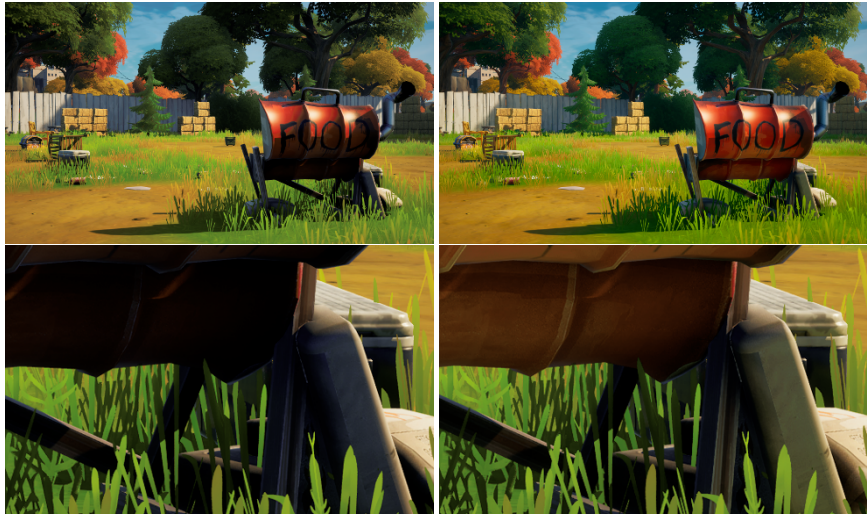
Figure 48-12. Fortnite's Risky Reels, before and after applying ray traced global illumination. Note the bounce lighting from the grass to the grill.
