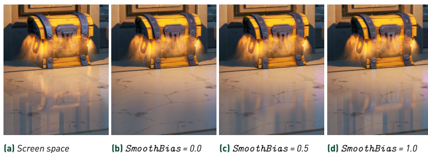
Figure 48-6. The visual effect of varying the smoothness bias.
