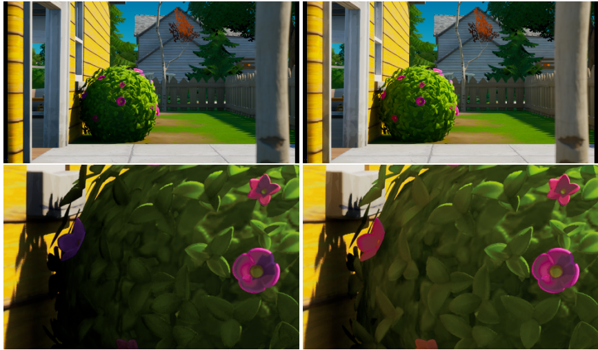
Figure 48-13. The brute-force global illumination technique in our development test environment, rendered with two samples per pixel at ScreenResolution = 50 . Note the yellow color bleeding from the nearby wall onto the bush.
