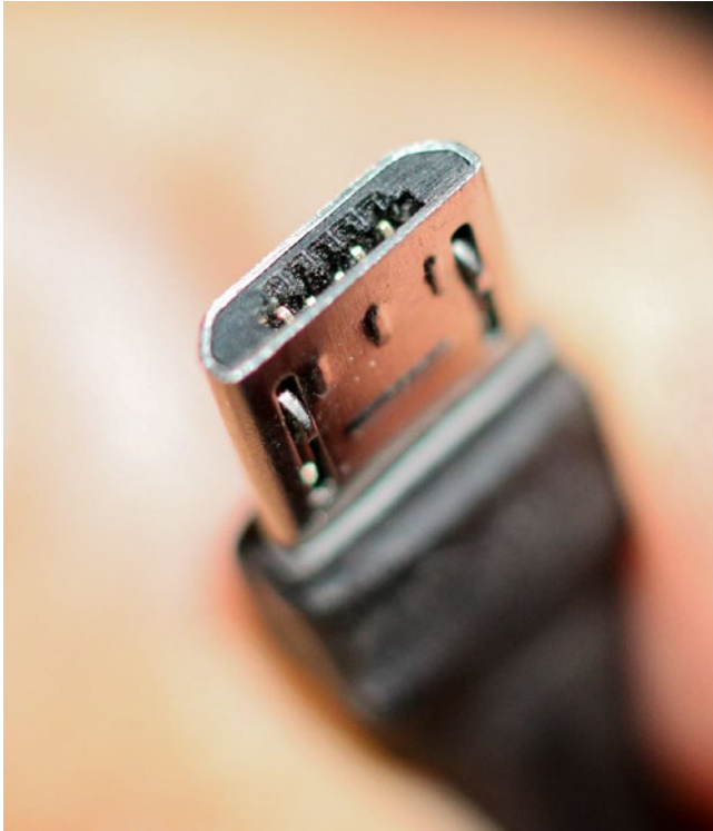
Figure 1-4. Micro-USB male pin
