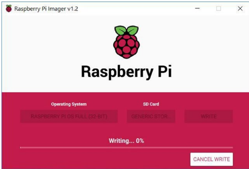
Figure 1-15. Writing the OS to the microSD card
