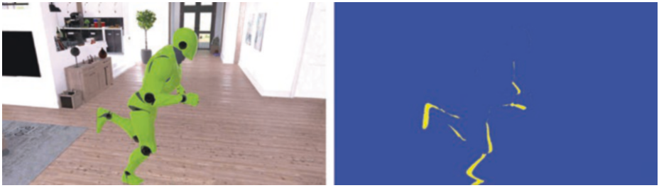
Figure 22-4. A skinned character in the middle of a run animation (left). Motion vectors are used to determine disocclusions that cause TAA to fail. TAA ghosting artifacts are eliminated and disocclusions are antialiased by marking these areas for ray traced supersampling (right).
