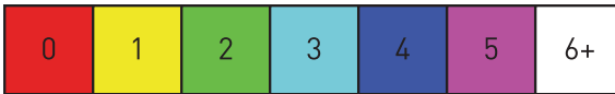
Figure 20-9. The mip level colors in the rainbow texture are selected according to this image, i.e., the bottom mip level (level 0) is red, level 1 is yellow, and so on. Mip levels 6 and above are white.
