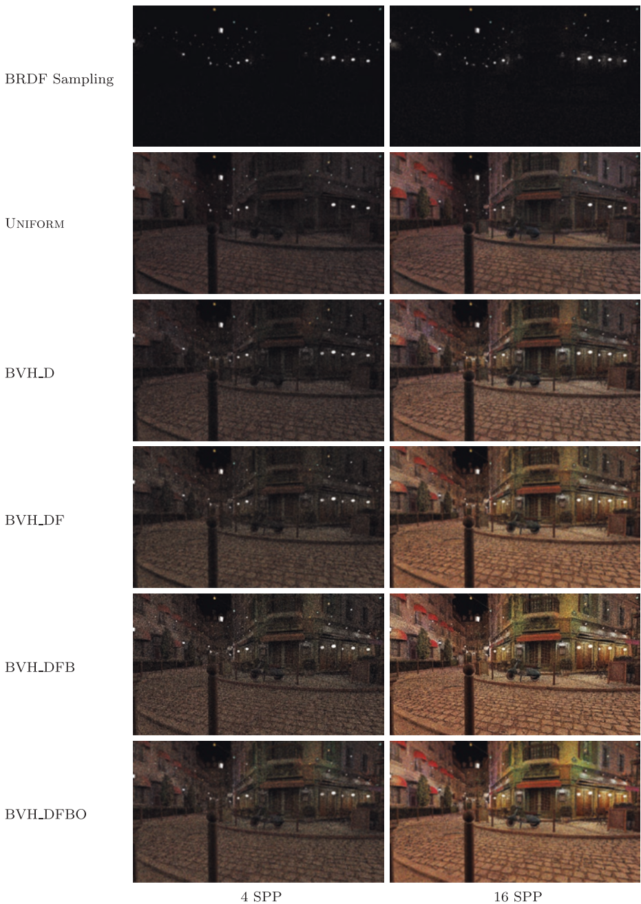
Figure 18-9. Visual results at 4 samples per pixel (SPP) (left) and 16 SPP (right), using the different sampling strategies defined in Section 18.4.3. All BVH-based methods use a BVH built with SAOH evaluated for 16 bins along all axes. The BVH techniques use MIS: half their samples sample the BRDF and half traverse the light acceleration structure.
