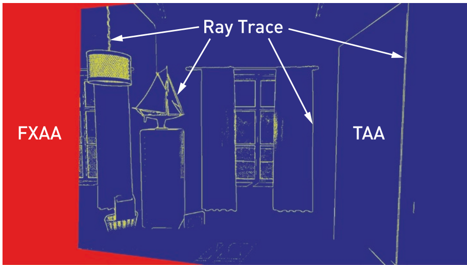
Figure 22-3. An annotated visualization of an ATAA segmentation mask. Blue pixels use standard TAA, red pixels use FXAA, and yellow pixels use ray traced supersampling.
