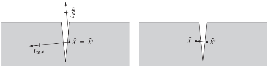
Figure 6-8. Very fine geometric detail such as a deep, thin crevice cannot be robustly handled by any of the listed methods. In this example the initial intersection \tilde{X} is slightly below the actual surface. Left: limiting the ray interval can help to avoid self-intersection for some rays (upper ray), but may also fail for others (lower ray). Right: offsetting along the surface normal may move the origin of the next ray \tilde{X}' into the same or neighboring object.
