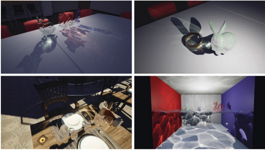
Figure 30-1. Caustics generated by screen-space photon mapping, with 2k \times 2k photons for each scene: from top left to bottom right, Conference Room, Ring and Bunny on Conference Room (Ring & Bunny), Bistro, and Cornell Box. Performance measures are shown later in Table 30-2.
