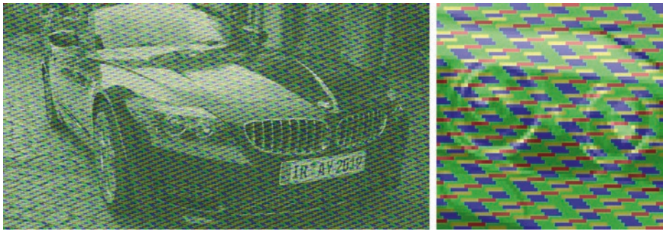
Figure 10-2. Adaptive tiling for four processing units with relative weights of 10% (red), 15% (yellow), 25% (blue), and 50% (green). Note how the headlight pixels are distributed among processing units.
