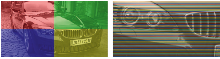
Figure 10-1. Left: uniform tiling with four processors. Right: detail view of scanline-based work distribution.
