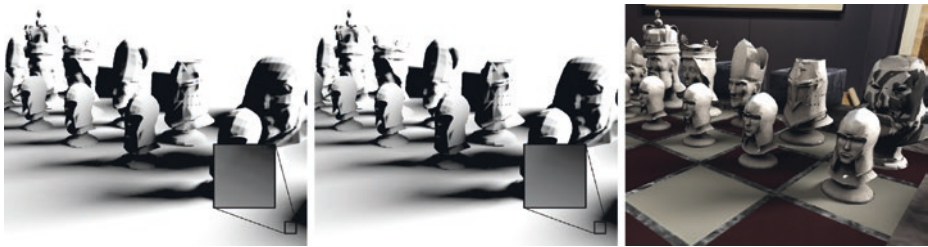
Figure 13-13. Difference between standard and high-quality adaptive sampling. Left: normal quality (up to 5 samples per pixel). Center: high quality (up to 8 samples per pixel). Right: final render using the high-quality setting.
