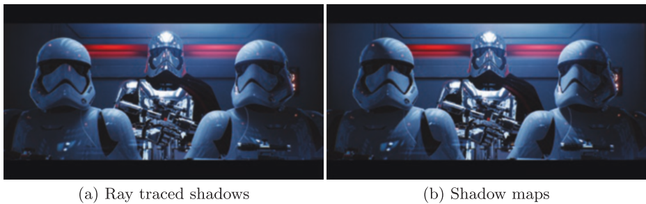
Figure 19-3. (a) Original rendering from the “Reflections” (Lucasfilm) demo with ray traced soft shadows. Notice the soft shadows under the helmet of the two stormtroopers. (b) Without soft shadows, the lighting loses the fidelity in the area light illumination, and the image is less photorealistic.
