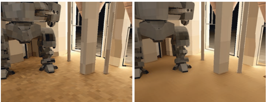
Figure 23-10. Left: light map data visualized after the merge and dilation operations. Right: light map data visualized after the denoiser step. In both pictures bilinear filtering is disabled to emphasize the noise reduction.
