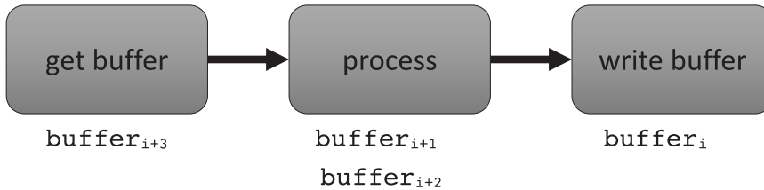
(a) A parallel filter can process more than one item in parallel.
