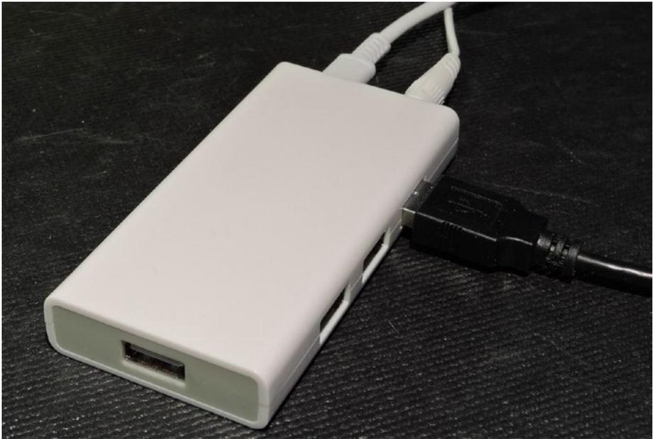
*Figure 7-1. A powered USB hub*
