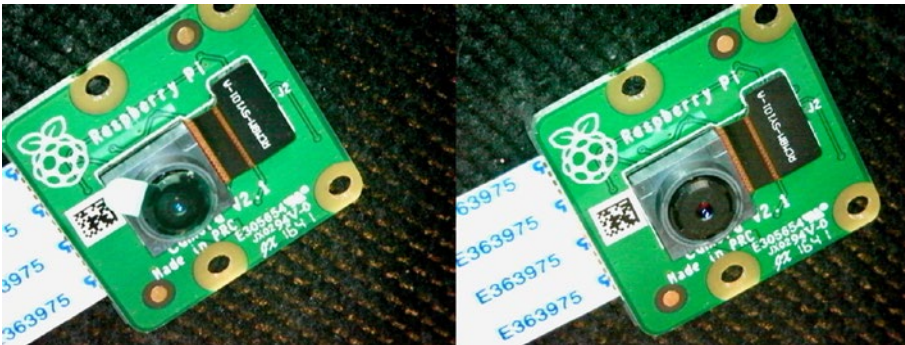
Figure 26-5. Camera with protective lens cover (left) and covering removed (right)
