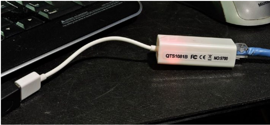
Figure 8-5. A wired USB ethernet adapter plugged into an USB extension cable
