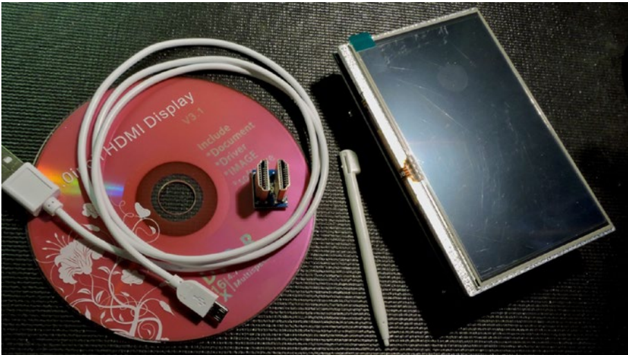
Figure 24-1. The 5 Inch HDMI Display kit with stylus, DVD, and LCD unit (with plastic covering still attached). USB power cable is not included.
