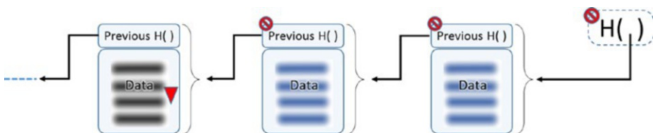
Figure 2-21. Any attempt in changing Header or Block content breaks the entire chain. Assume that you altered the data in block-1234. If you do so, the hash that is stored in the block header of block-1235 would not match.
