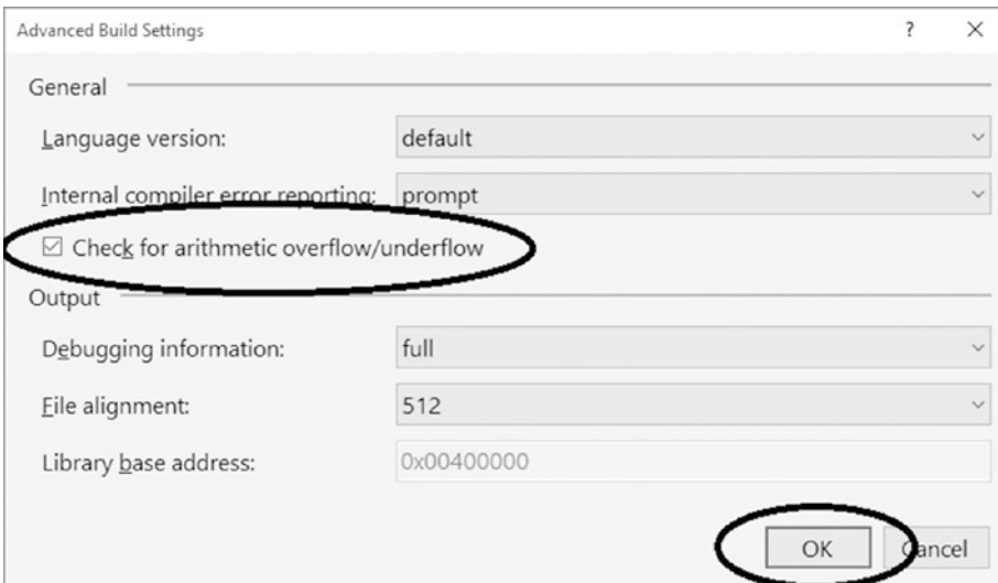
Figure 12-6. “Check for arithmetic overflow/underflow” check box
