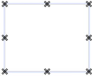
Figure 31-13. A locked object is indicated by a restriction icon in place of sizing handles
