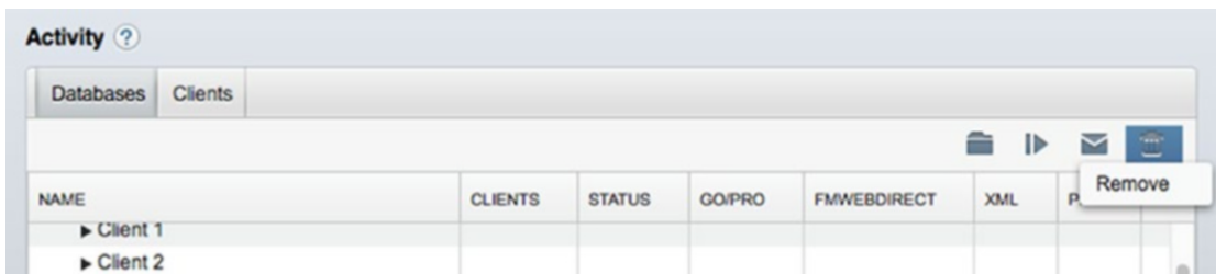
Figure 39-10. The Remove option is used to safely remove files from the list of available databases and place them into a subfolder of the Databases folder for moving and copying elsewhere
