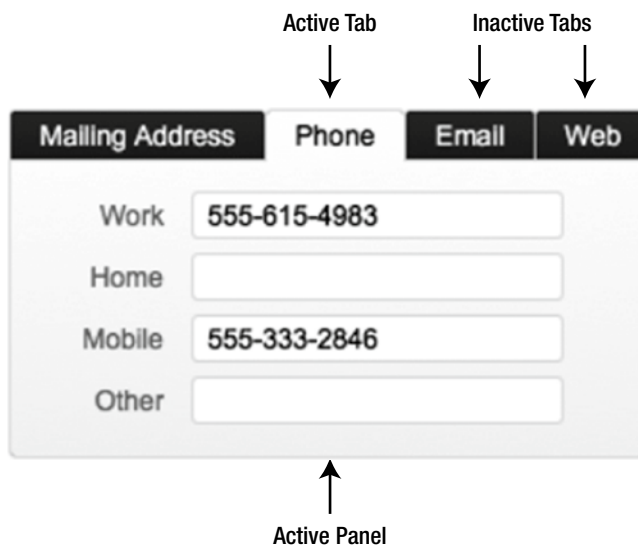
Figure 30-47. An example of a tab control with four tabs, actively displaying the second tab
