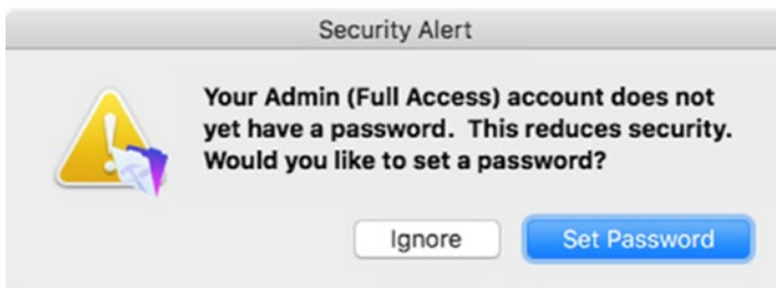
Figure 40-1. A dialog warning about the lack of a password on the default full access account named Admin
