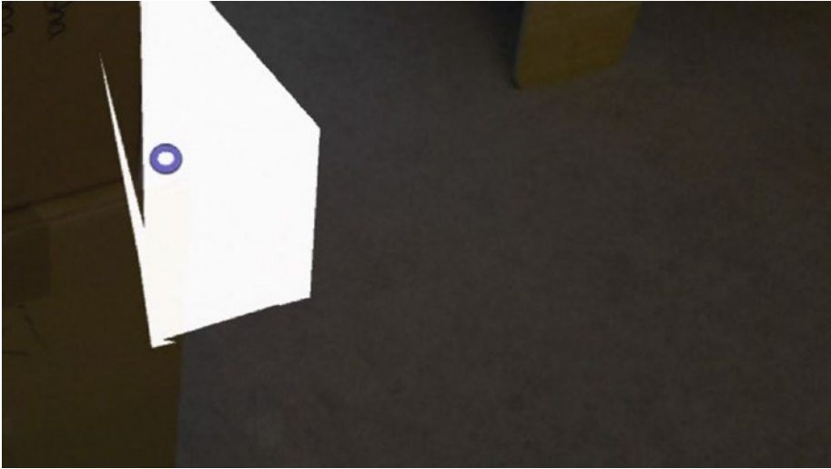
Figure 6-15. When obstructed (in this case by boxes), only the unobstructed part of the cube is visible
