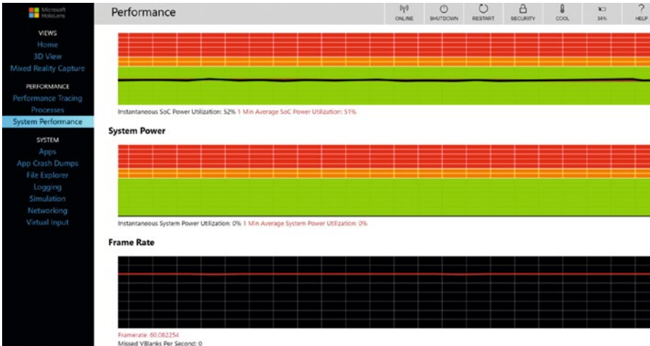
Figure 8-2. You can track real-time performance metrics for the HoloLens via the Windows Device Portal
