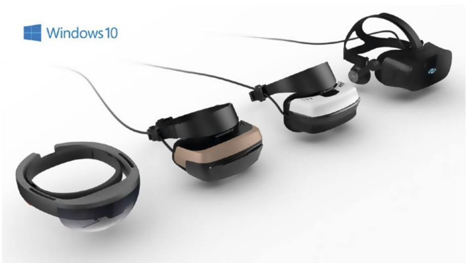
Figure 1-6. Examples of Windows Mixed Reality devices include both transparent headsets such as the HoloLens and immersive headsets (source: Microsoft)
