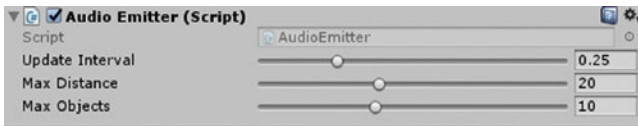
Figure 7-7. Adjustable parameters of the AudioEmitter.cs script, as seen in the Inspector panel of Unity’s Editor
