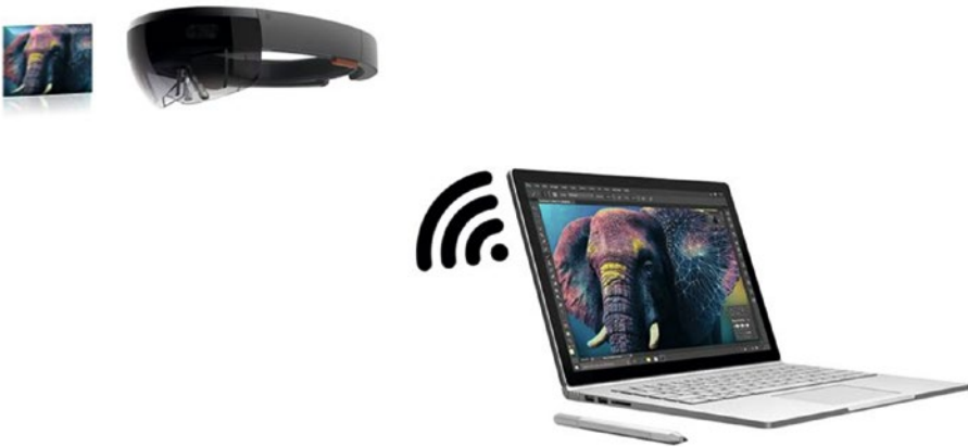
Figure 1-1. Illustration of holographic remoting. The PC streams the app to the HoloLens for viewing, without the need to install the test app on the HoloLens.
