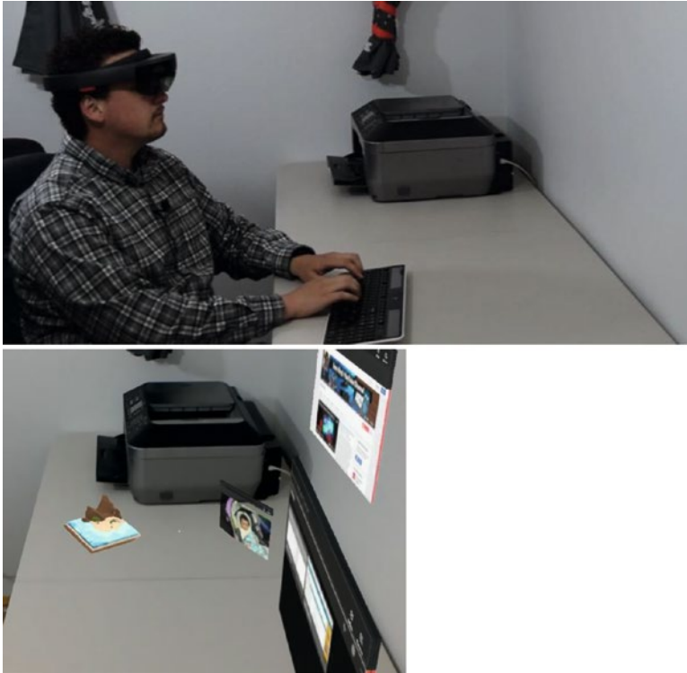
Figure I-1. The HoloLens enables an empty desk (top image) to be filled with holographic computer monitors and desk decorations (bottom image)
