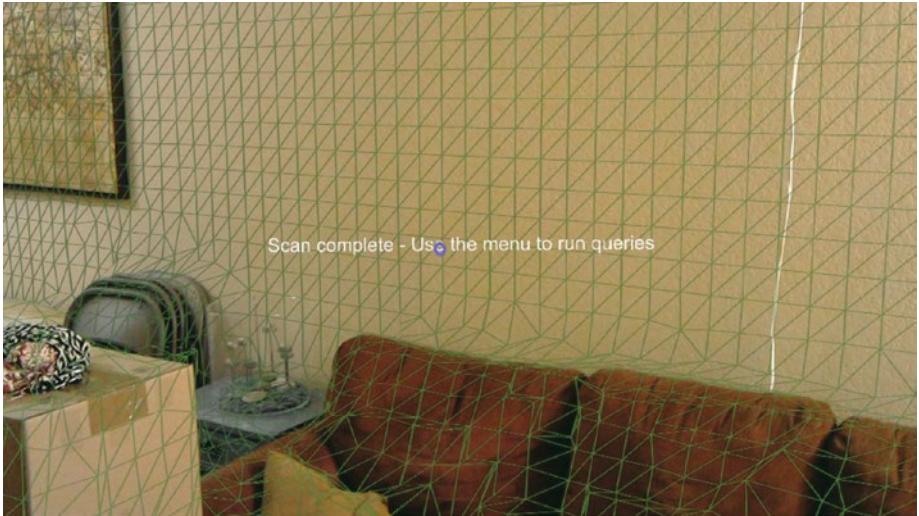
Figure 6-17. The spatial mapping mesh processing by spatial understanding is remarkably smooth
