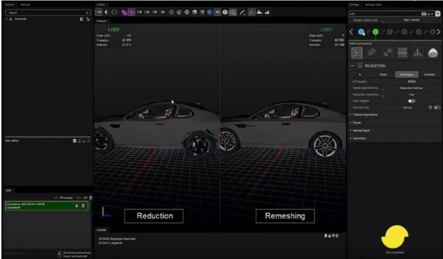
Figure 8-9. Simplygon allows you to convert large, complex 3D models into beautiful, low-poly models that performs well in the HoloLens
