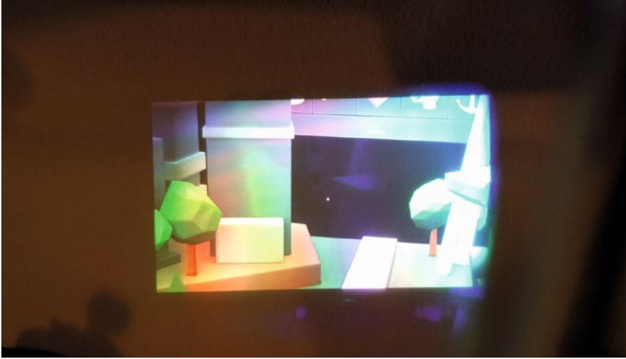
Figure 1-7. HoloLens field-of-view limitation, photographed from behind the device
