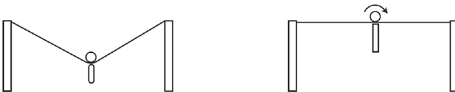
Figure 6-4. Problems with a heavy bot on a string (left image) or a motor that spins so fast that the bot doesn't move on the string (right image)
