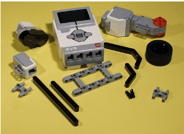
Figure 1-3. LEGO MINDSTORMS EV3 Intelligent Brick, motor, sensors, and other LEGO Technic components
