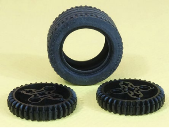
Figure 7-19. For the hub, use these two gears instead. They make a stronger connection to your axles and reinforcement parts.
