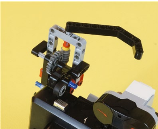
Figure 12-20. This Angle Crank lets you move up or down, to precisely position the camera shutter arm with its small rubber wheel
