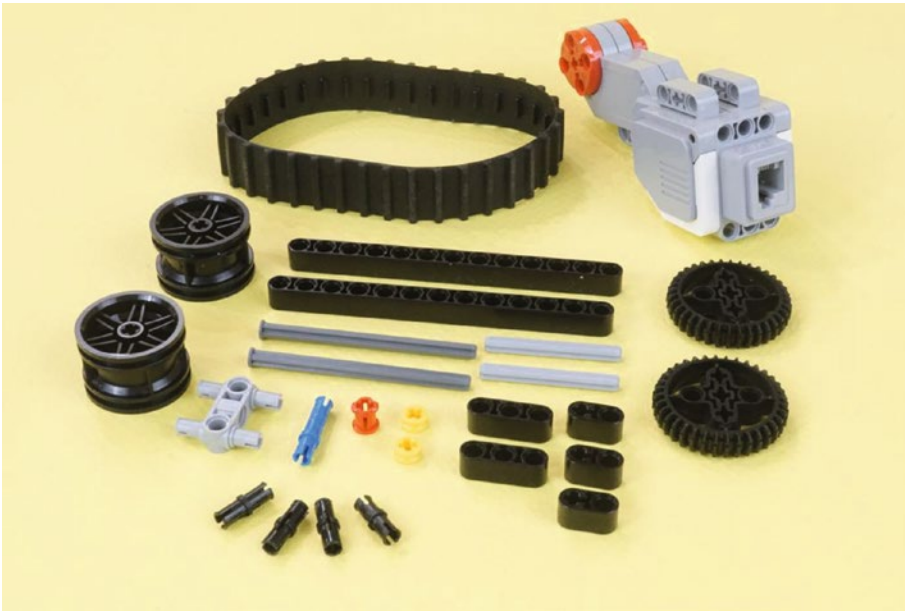
Figure 15-2. All of the components for one of the main body's tank-tread motor assemblies. You'll build two of these. Nail head axles are 8-hole. Gray axles are 5-hole.
