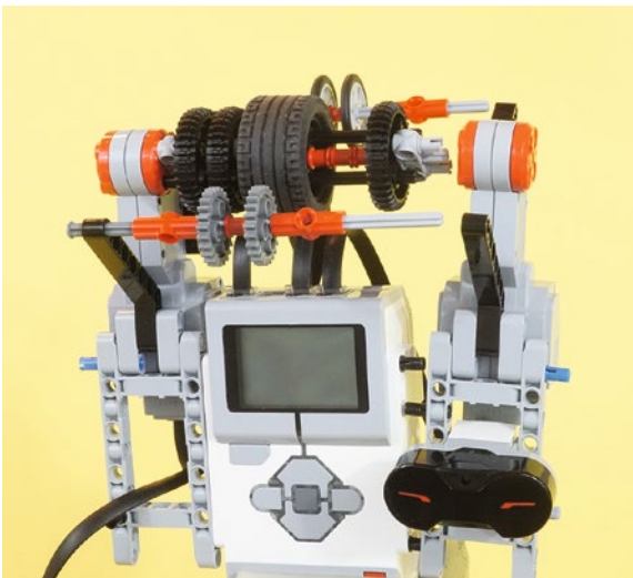
Figure 8-23. The StringBot can be “opened” to place the bot on a string, rather than threading the string through. (Red 11-beam removed to allow the assembly to separate.)
