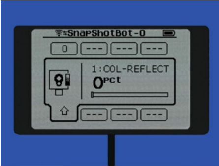
Figure 10-6. The Color Sensor screen in the COL-REFLECT mode
