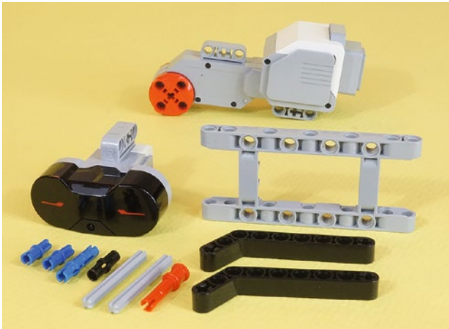
Figure 7-2. All the pieces for the StringBot right-side motor assembly with IR sensor. The axles are five holes in length.
