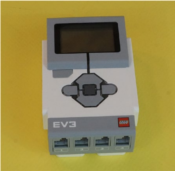
Figure 3-7. The body will consist of the Intelligent Brick, with motors and assemblies to be fastened to it
