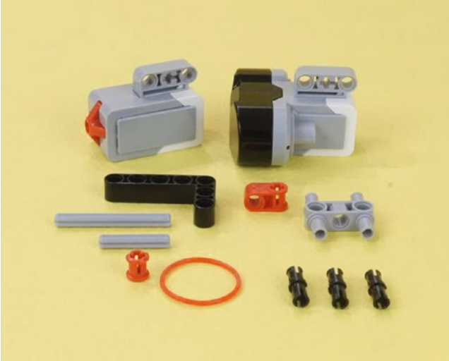
Figure 15-46. All of the remaining parts (axles are 3 and 5-hole) needed to mount the Touch and Infrared Sensors. There is also a Grabber Latch assembly, discussed next. These parts will take you all the way through Figure 15-52.
