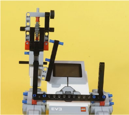
Figure 11-32. Preparing to attach the medium motor Camera Trigger assembly. Position the assembly on the hardpoint and slide the axle through first. Then fasten the 9-hole beam with connectors. It may be necessary to twist the short half-axle to make it fit into the motor.
