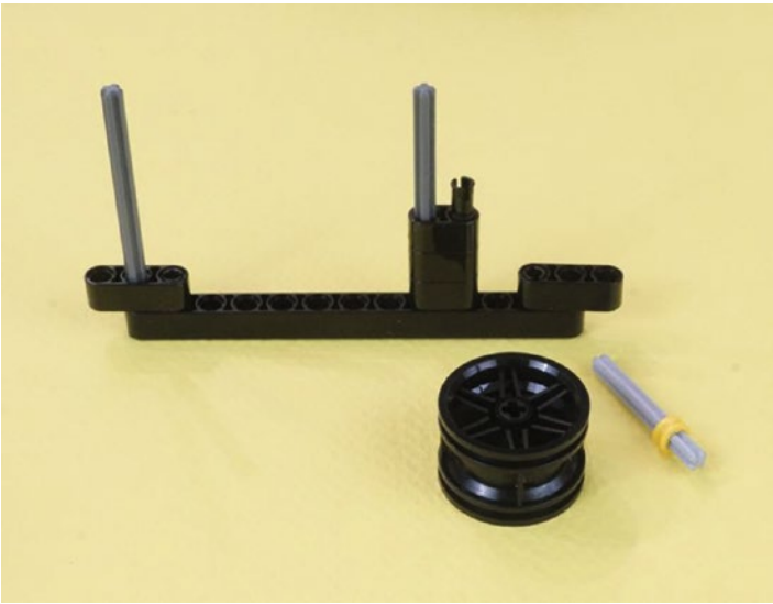
Figure 15-6. Push the long axles all the way in and set the unit on its side. In this picture, the unit was turned around the other way from Figure 15-5. The hub, short axle, and yellow collar join the scene.
