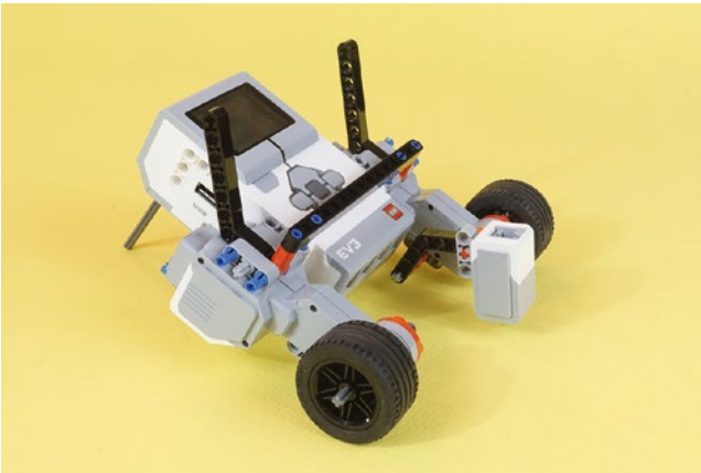
Figure 11-11. The Color Sensor assembly mounts to the center axle hole on the right motor. It is quite close to the floor, without touching.
