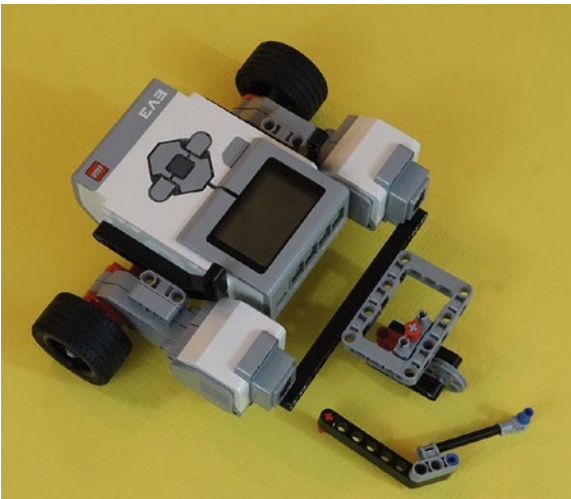
Figure 3-29. Rear-wheel reinforcement strut ready for installation between body and rear-wheel/base
