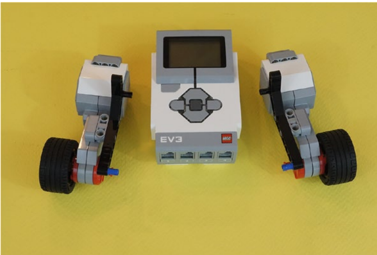
Figure 3-12. The Intelligent Brick and the motor/wheel combinations, before putting them together
