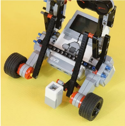
Figure 11-36. Swing each 15-hole beam up to meet the end of the angle beam. Keeping the red collar in place, fasten this together with the short nailhead axle.
