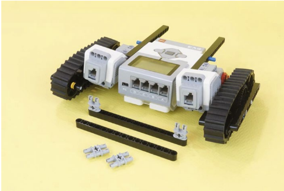
Figure 15-16. New parts—four dual-connectors and two 15-hole beams. Assemble them as shown in Figure 15-17.
