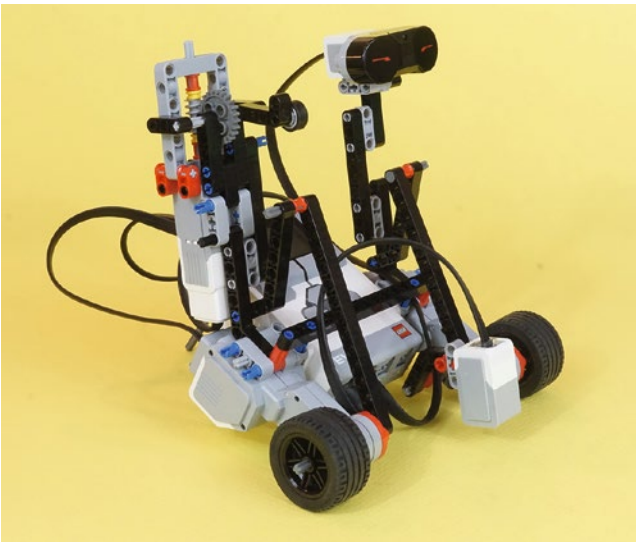
Figure 11-42. The completed, wired SnapShotBot, Camera Trigger assembly, front-side view
