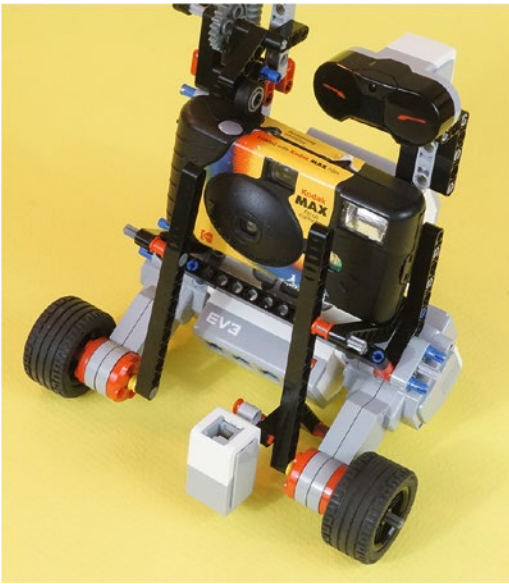
Figure 11-38. Move the 15-hole beams to a different position to accommodate this larger disposable camera. The angle pieces bend down, allowing a different point of connection. In this case, a longer lever would be needed for the shutter lever wheel to reach this camera's shutter.
