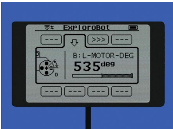
Figure 4-24. Observing how many degrees the motor on port B rotates, with the ExploroBot turned 90 degrees by hand
