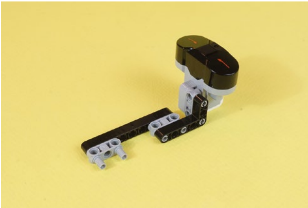
Figure 11-14. The IR Sensor assembly, ready to be mounted. Set it aside for now or mount it as shown in Figure 11-33.
