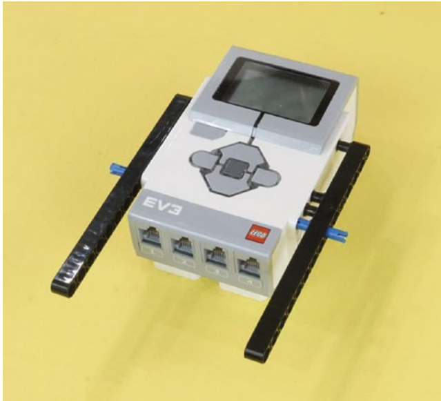
Figure 15-13. The two 15-hole beams being attached to the Brick
