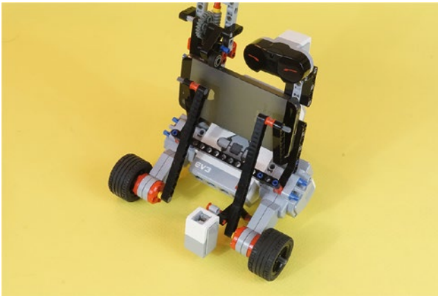
Figure 11-37. With the original design, this SnapShotBot supports a smartphone camera. This type of smartphone will take a picture when the shutter lever wheel presses its side button. The lens is at the lower left of the phone and can see past the beams.
