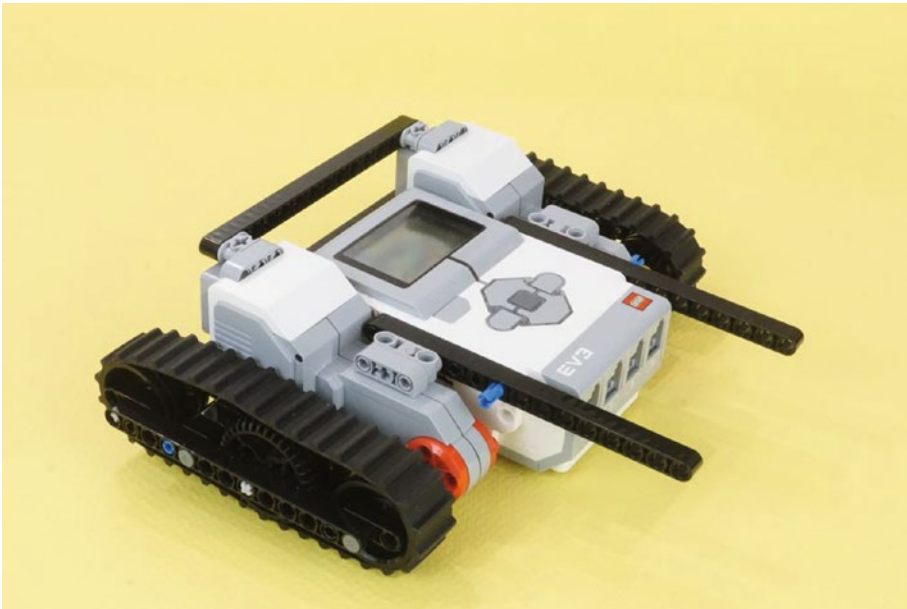
Figure 15-18. Another view of the tank driving base. This is an excellent driving base for other projects. It rides rather low, but is very stable.
