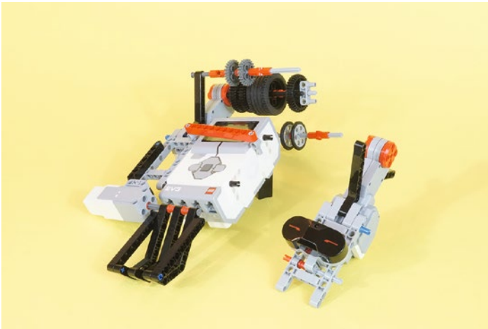
Figure 7-42. It’s starting to look like a StringBot. The front reinforcement 11-beam goes on last; it’s shown for completeness.
