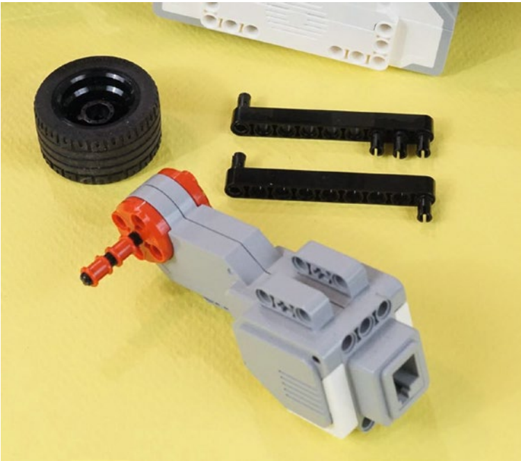
Figure 19-62. The axle goes into the large motor, along with two collars. Press the tire onto the axle. Put the six pins into the two nine-hole beams.
