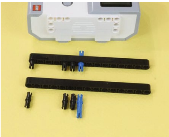
Figure 15-12. New parts. Two 15-hole beams with four pins apiece.
