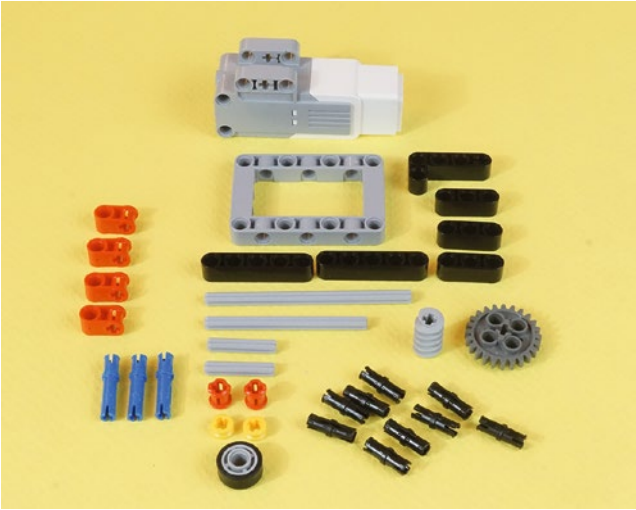
Figure 11-15. All of the parts for the medium motor Camera Trigger assembly. These parts will take you up through Figure 11-28.
