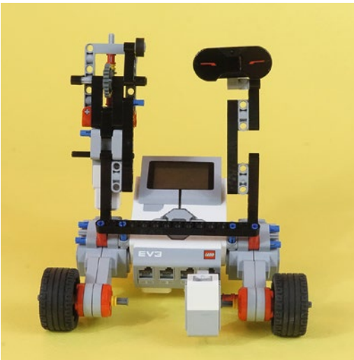
Figure 11-33. The medium motor Camera Trigger assembly is now attached to the body. Snap the IR Sensor assembly in as shown on the right.
