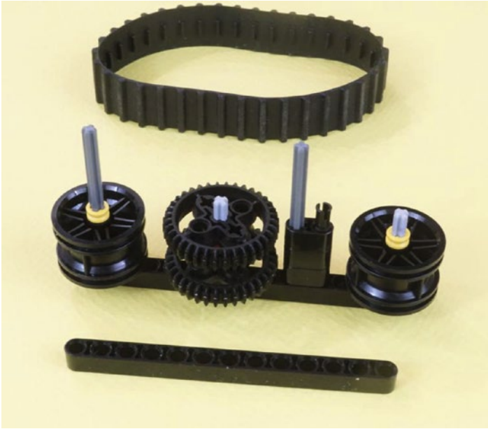
Figure 15-8. The second hub and the gear-wheel assembly are in place. The remaining 13-hole beam is ready to be mounted. The single black pin in the center will keep the beam from falling off. Mount the beam so all three axles go through. Then stretch the tank-tread over the end hubs.
