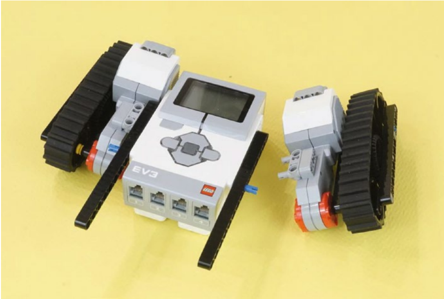
Figure 15-14. The Brick and tank-tread motor assemblies give us the main body. One is connected, the other is ready to go.
