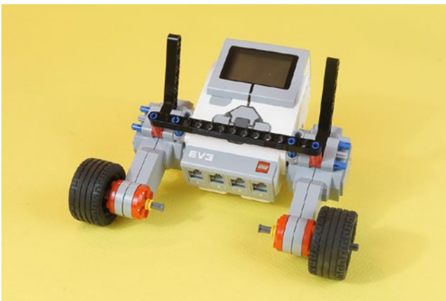
Figure 11-8. The basic body, with hardpoints
