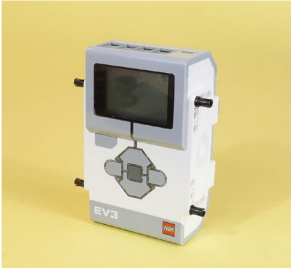
Figure 7-40. The Intelligent Brick makes its appearance! Connectors go into the outer four corners
