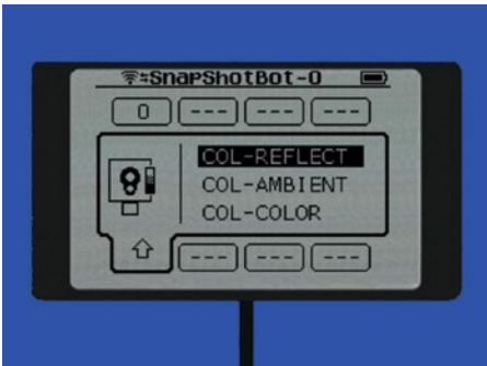
Figure 10-7. Selecting the COL-REFLECT mode
