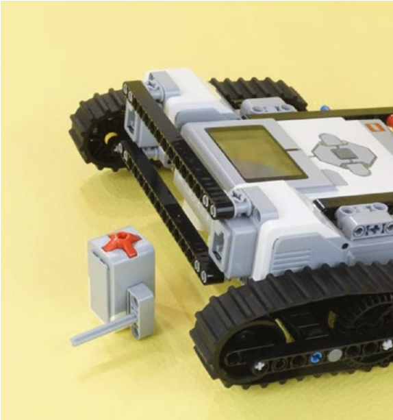
Figure 15-50. The Touch Sensor axle goes in the center Touch Sensor axle-hole. It mounts to the Tank Drive Base, as shown in Figure 15-51.
