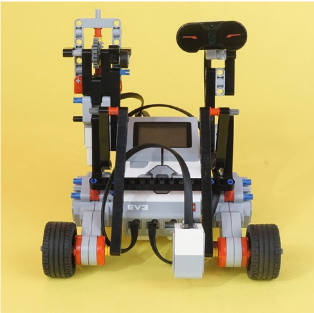
Figure 11-46. The completed, wired SnapShotBot, front view. This is a good view of the sensor wires. The Color Sensor is in port 1. The IR Sensor is in port 2.
