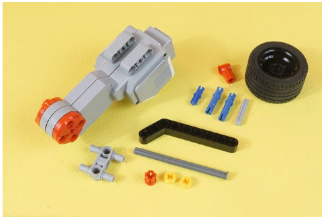
Figure 11-2. Starting pieces for one of the SnapShotBot's motors. The two motor assemblies are mirror images, starting with identical parts. So you'll need twice the number of parts shown in this figure to build both motors.
