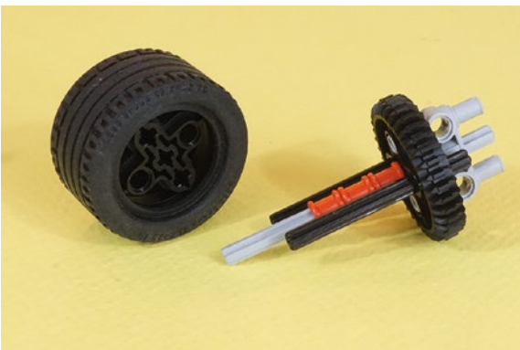
Figure 7-23. Another view of the three-axle gear assembly, about to be inserted into the three axle-holes of the tire
