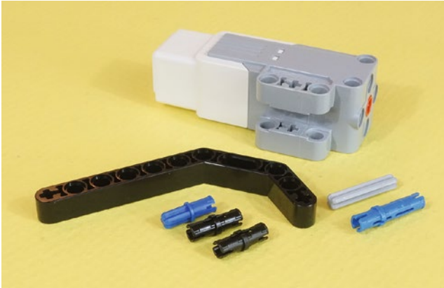
Figure 7-35. All the parts for the motor frame. The axle is a three-hole length type.
