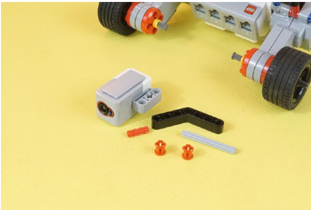
Figure 11-9. Here are the parts needed to mount the Color Sensor
