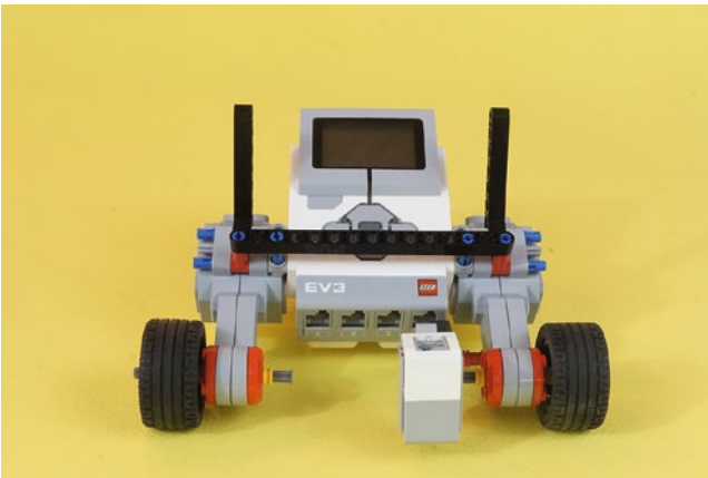
Figure 11-12. Another view of the Color Sensor assembly, mounted in place
