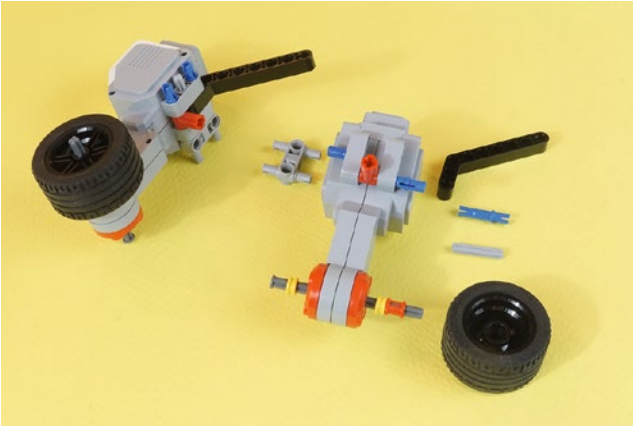
Figure 11-3. Using the duplicate sets of parts from Figure 11-2, assemble the right and left sides. Notice that the long axle is a nailhead. The heads will be facing the center.
