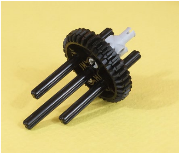
Figure 7-25. Now make this similar three-axle assembly for the other side, using the fourth gear. No red collars on this one.
