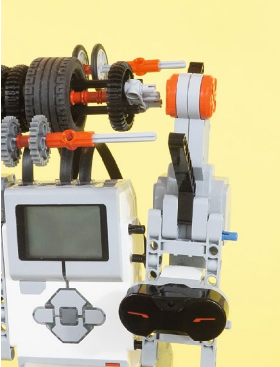
Figure 7-44. The right-side motor clips on to your StringBot
