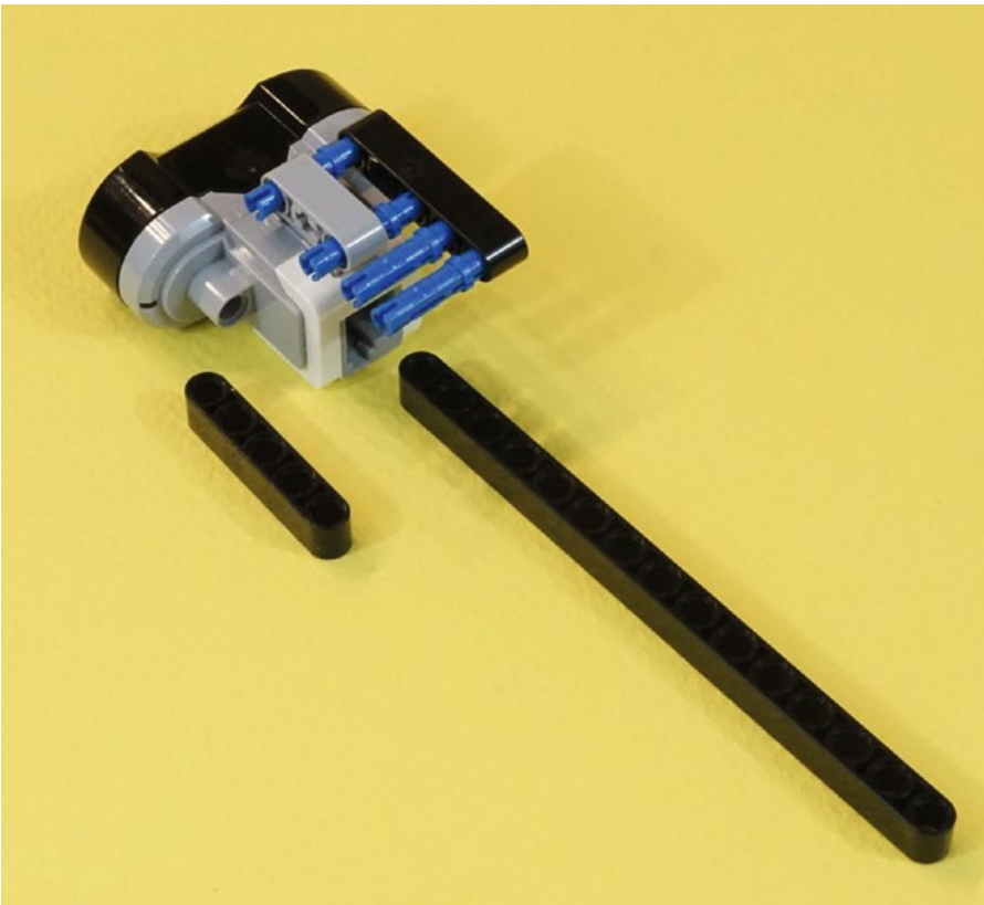
Figure 19-39. Begin the assembly of the head. These four connectors will fasten the two five-hole beams to the 15-hole beam.
