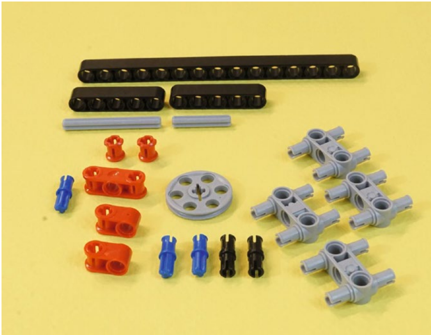
Figure 19-28. These are all of the parts you need for this section. You'll have the caster wheel and an important part of the frame. The axles are five-hole and three-hole lengths.
