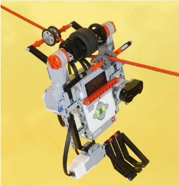
Figure 8-22. The string passes through the rear string guide, around the rubber tire, and out the front guide
