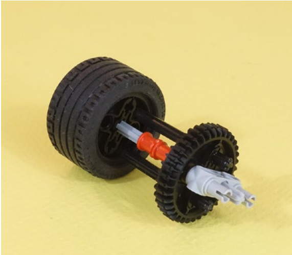
Figure 7-24. The three-axle assembly partially inserted. Push it in until the collars stop it.
