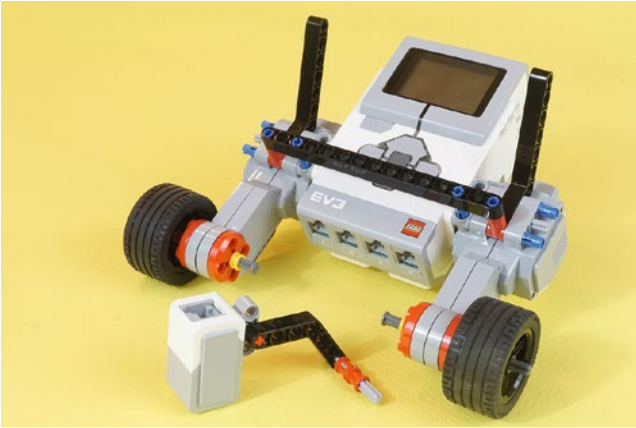
Figure 11-10. The Color Sensor assembly
