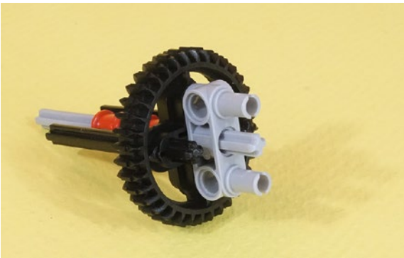
Figure 7-22. When the gray connector is seated, the axle should be level with the gray pins
