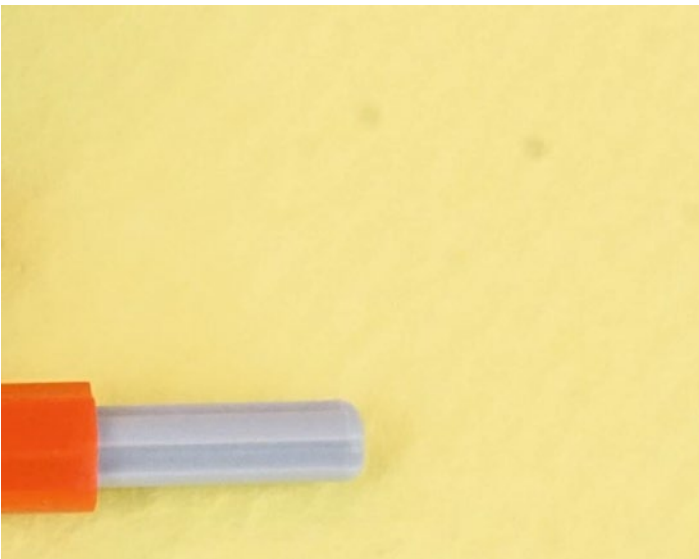
Figure D-4. Enlargement of Figure D-3. What are those little gray dots doing there? Very possibly, they're dust on the sensor.
