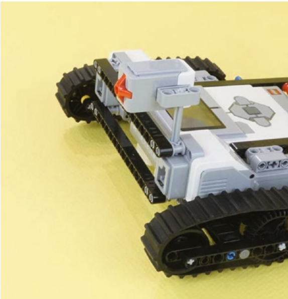
Figure 15-51. A convenient place to mount the Touch Sensor is in the double connector holding the 15-hole beam in place. This single point of attachment is sturdy enough to let the Touch Sensor be used as a Start switch.
