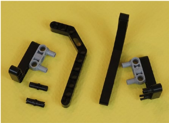
Figure 3-3. Beginning assembly of the parts for the left and right sides of the neck that will hold the ExploroBot's head
