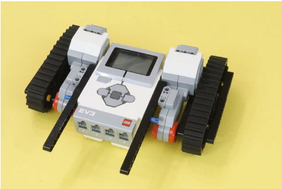
Figure 15-15. Both tank-tread motor assemblies in position
