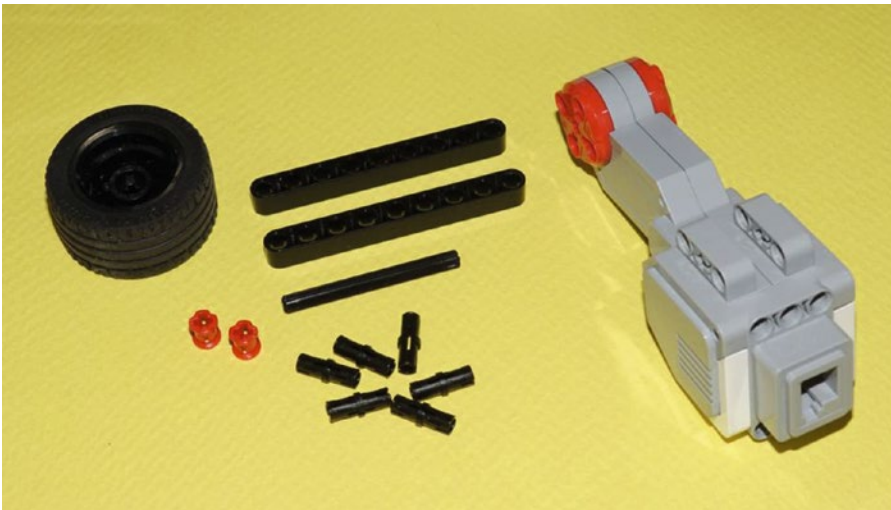
Figure 19-61. All the parts to make one large motor drive wheel assembly. You'll make two of these, as mirror images. The axle is a six-hole length.
