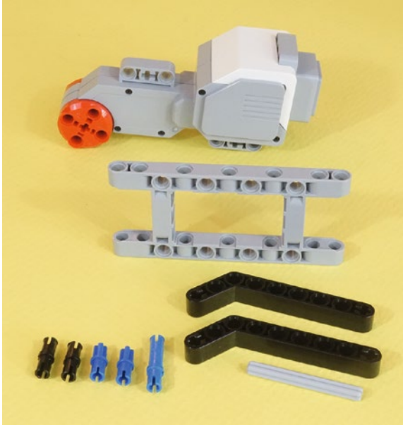
Figure 7-12. These are all of the parts for this sub-assembly. These axles are the kind with five-hole length.
