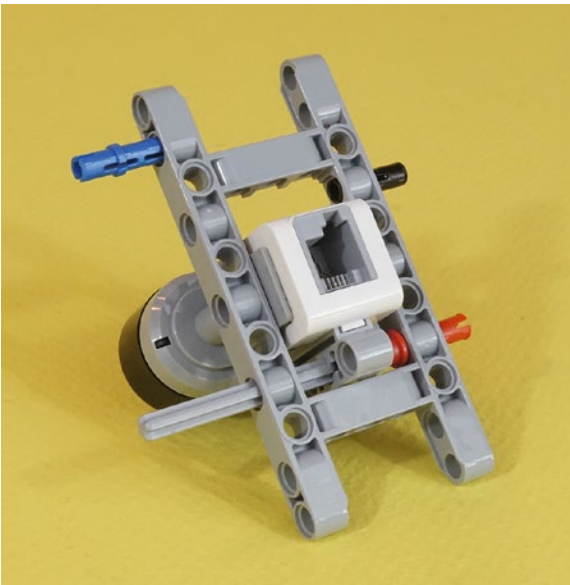
Figure 7-5. The axle engages the sensor in its middle axle-hole, then is seated in the red connector
