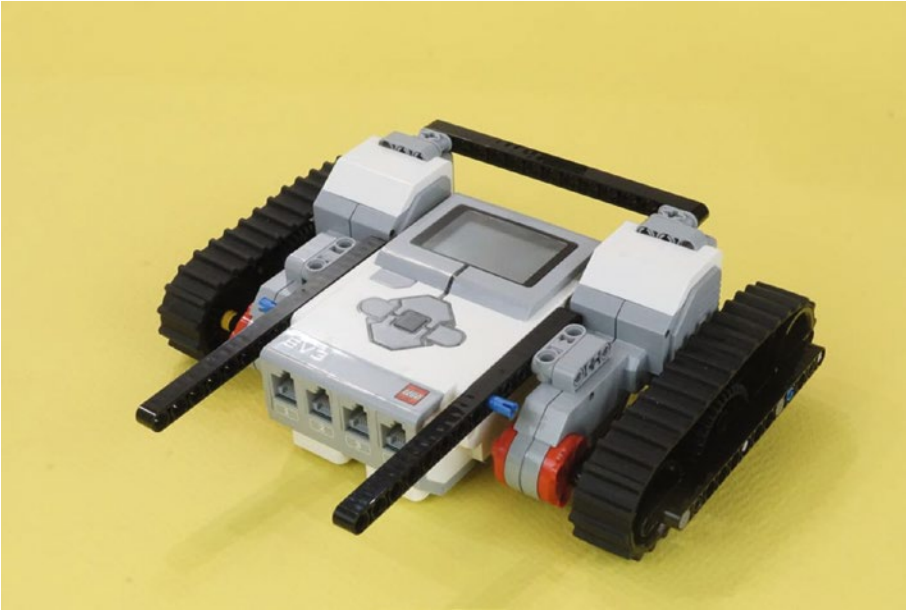
Figure 15-19. And one more view of the tank driving base. The two beams extending forward are excellent hardpoints for any project. The protruding blue pins are there just in case they will be useful as attachments.
