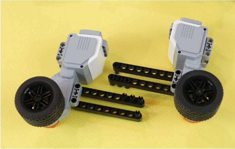
Figure 19-64. Both of the motors with frame pieces, ready to be attached to the Brick
