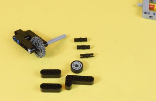
Figure 11-20. Still more parts from Figure 11-15. Now for the actual trigger mechanism and 3-hole beam side fasteners that will secure it to the Worm Gear sub-assembly.
