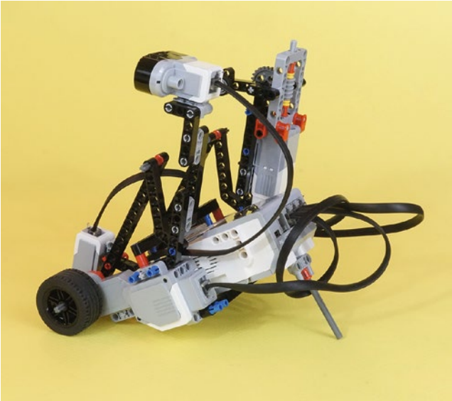
Figure 11-45. The completed, wired SnapShotBot, IR Sensor rear-side view
