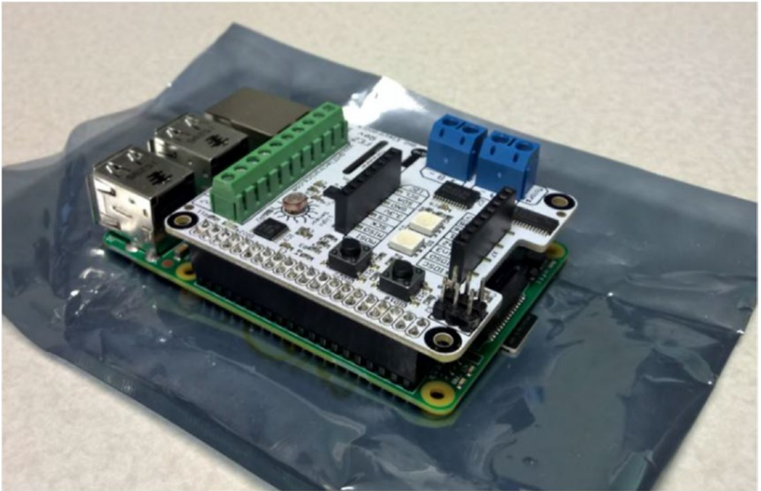
Figure 2-14. FEZ HAT with a Raspberry Pi
