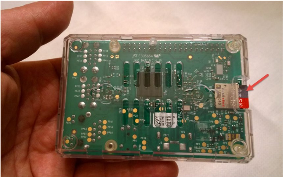
Figure 2-3. Inserting the MicroSD card into the Raspberry Pi
