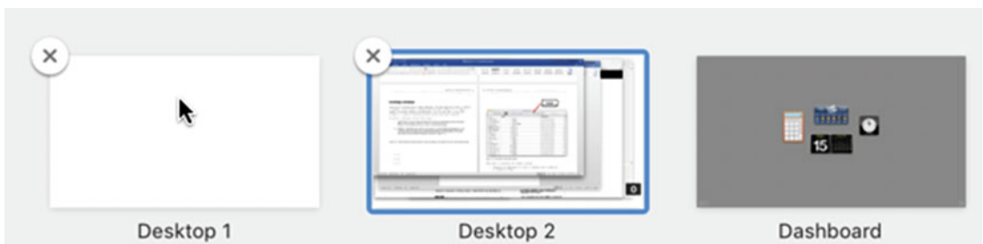
Figure 12-11. When holding the Option key down, a close button appears in the upper-left corner of each desktop image
