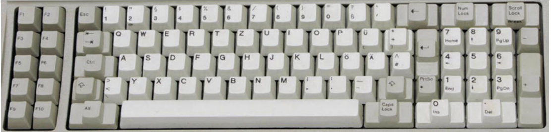
Figure 1-1. The keyboard of the original IBM PC combined cursor keys with a numeric keypad
