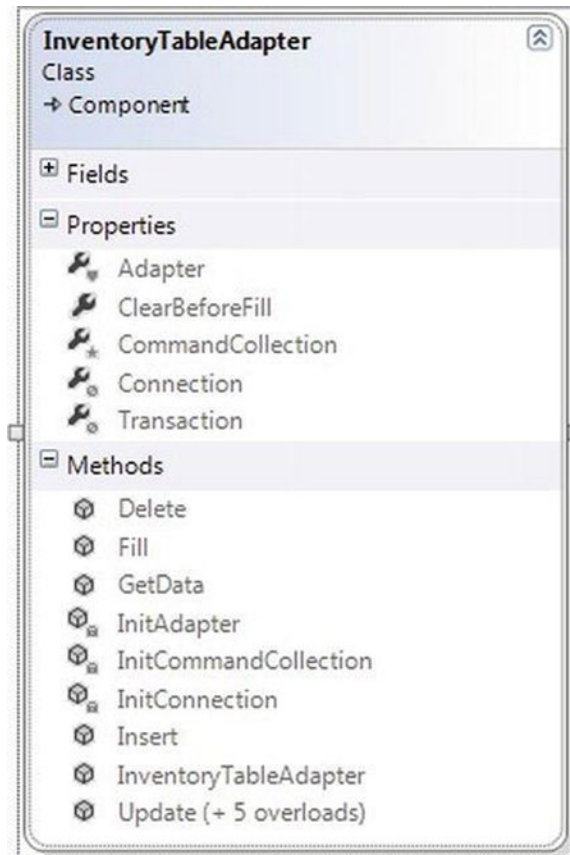
Figure 22-24. A customized data adapter that operates on the strongly typed DataSet and DataTable
