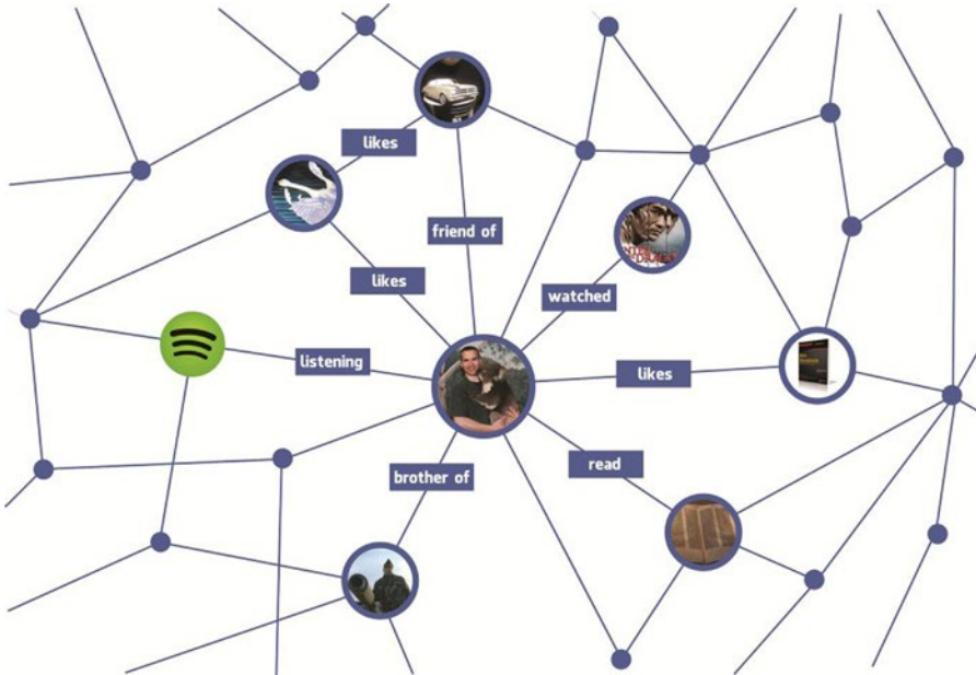
Figure 8-4. On the Facebook Social Graph, every object is a node and every connection is an edge
