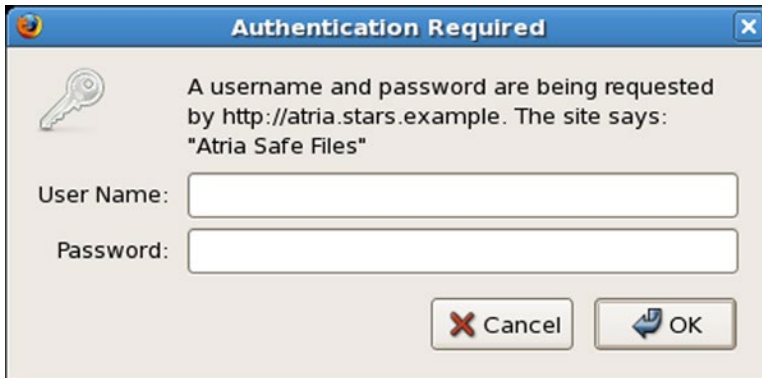
Figure 11-2. An Example of a Basic Authentication Request by Firefox 3.0.5 on CentOS 5.3
