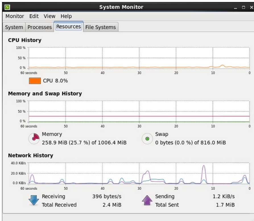
Figure 13-14. A view of the system monitor on a CentOS 6.5 (x86) system under active Slowloris attack
