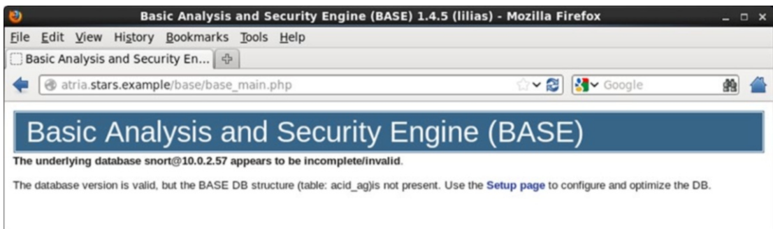
Figure 18-3. The BASE application, immediately after installation using a database that has not been prepared for BASE. Shown on CentOS 6.5
