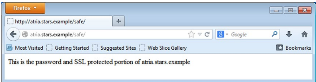
Figure 13-6. View of an SSL/TLS protected web site that has been intercepted by Ettercap and sslstrip. Note that the address bar shows no errors, and only the tab title shows that it is using http instead of https. Firefox 22 on Windows 7
