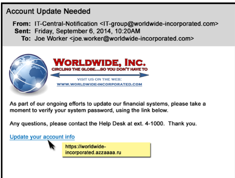
Figure I-3. Joe instead sees that the hyperlink would take him to a malicious domain
