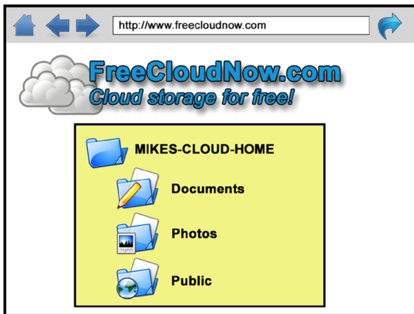
Figure 3-1. Most cloud storage services include (by default) a number of subfolders. One or more of these folders may be publicly accessible to the world at large. Users should take care when storing files in the public folder, and ensure that private/proprietary data are not stored there.
