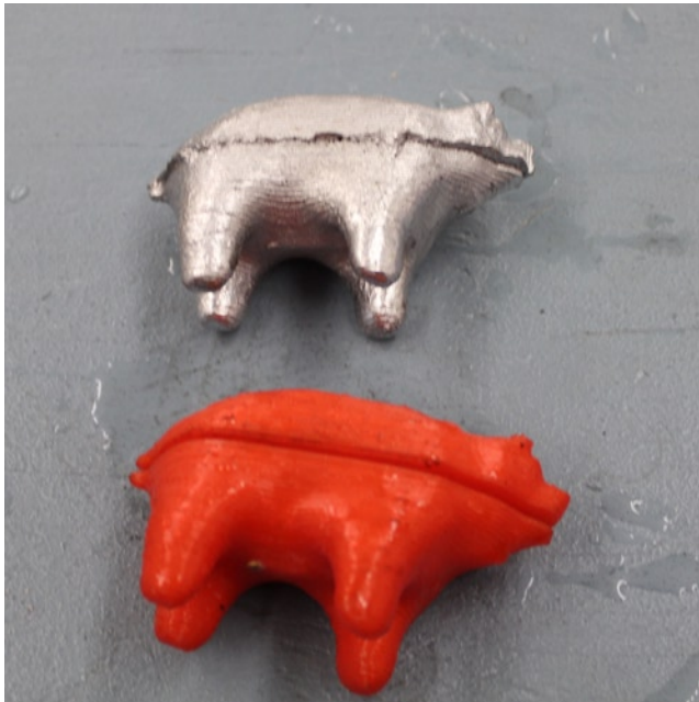
Figure 9-20. The bear, cut in half in PLA (two pieces) and aluminum (one piece)
