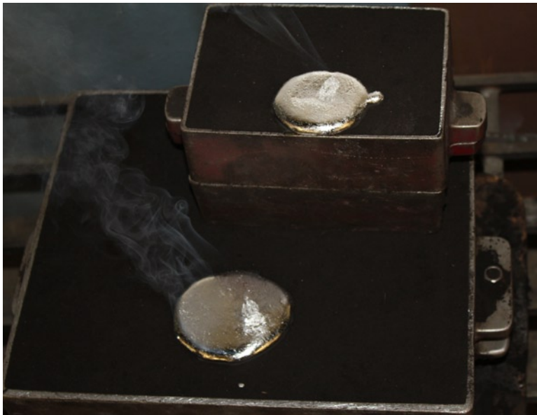
Figure 9-16. Two flasks with molten aluminum cooling
