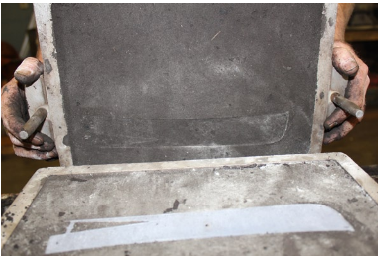
Figure 9-11. The pattern and its impression on the top half of the mold
