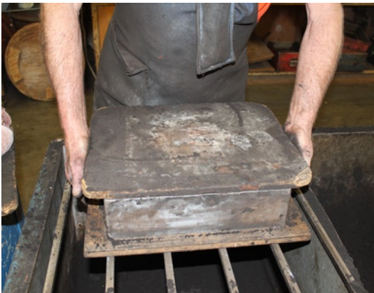
Figure 9-7. Getting ready to flip the flask upside-down
