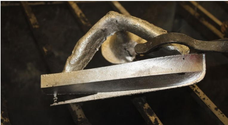
Figure 9-18. The boat and its sprues
