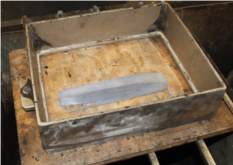
Figure 9-3. The boat pattern in the flask
