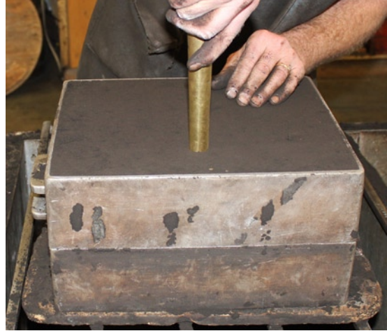
Figure 9-13. Making a good, clean, circular hole
