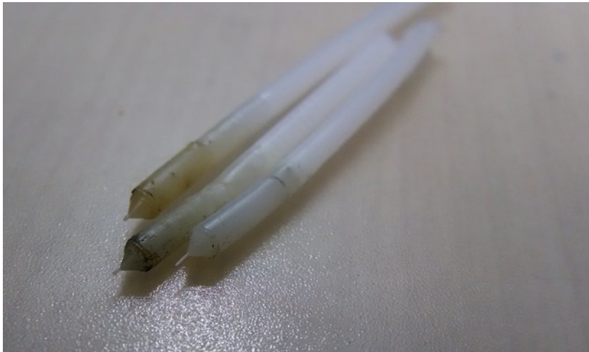
Figure 11-5. Nylon with residue of overheated plastic
