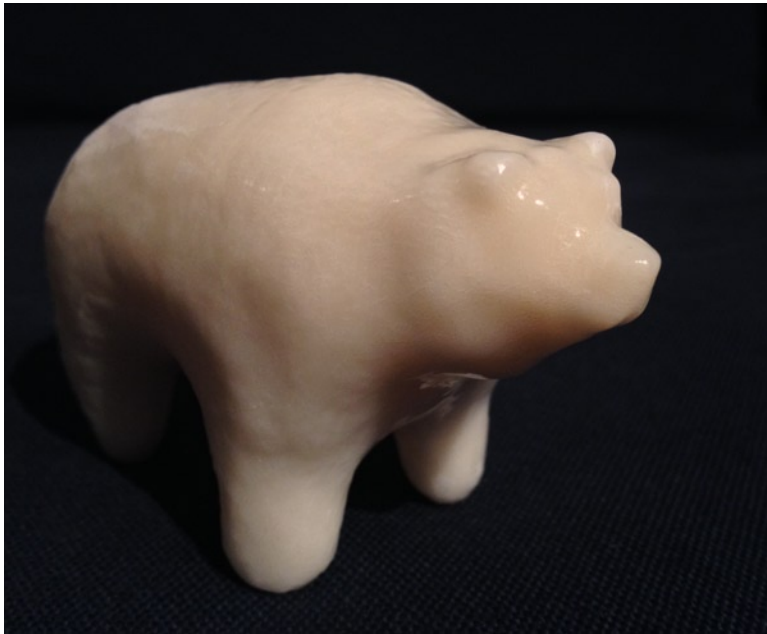
Figure 10-2. The Leopold bear from previous chapters, smoothed with acetone (front view)
