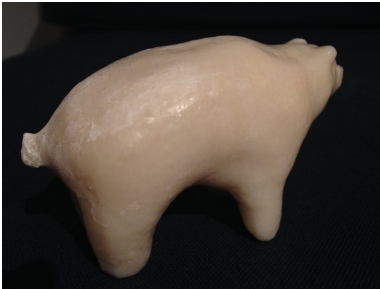
Figure 10-3. The Leopold bear from previous chapters, smoothed with acetone (rear view)
