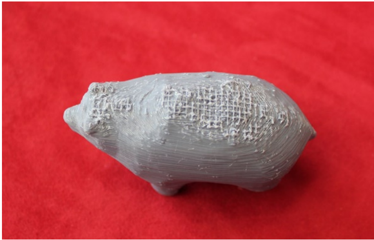
Figure 5-4. The same model from Figure 5-3, showing the scarring issues
