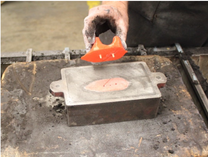
Figure 9-15. Setting up a part to be cast from a two-piece pattern
