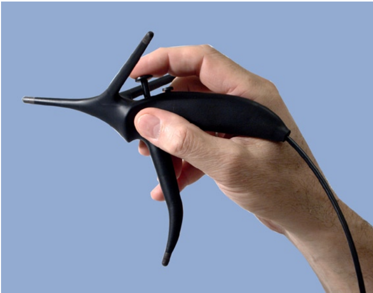
Figure 4-7. The Leonar3do bird input device. Photo courtesy of Leonar3Do International Plc
