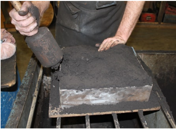
Figure 9-5. The bench rammer packs the sand around the pattern
