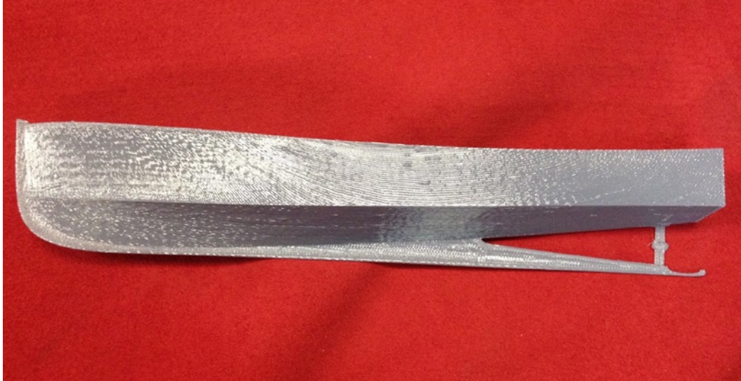
Figure 12-6. 3D-printed half hull of William Hand, Jr. boat. Created by Diego Porqueras from original design plans with permission from the Hart Nautical Collections of the MIT Museum. PLA print, hand-sanded
