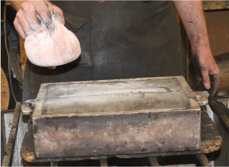
Figure 9-9. Using parting compound on the “bottom” of the pattern
