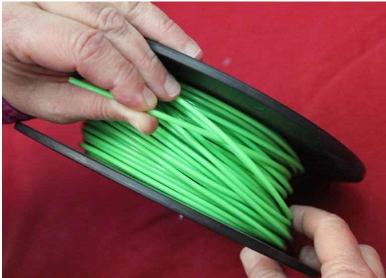
Figure 7-4. The wrong way to lay out filament at the start of the print (crossing a loop under another)
