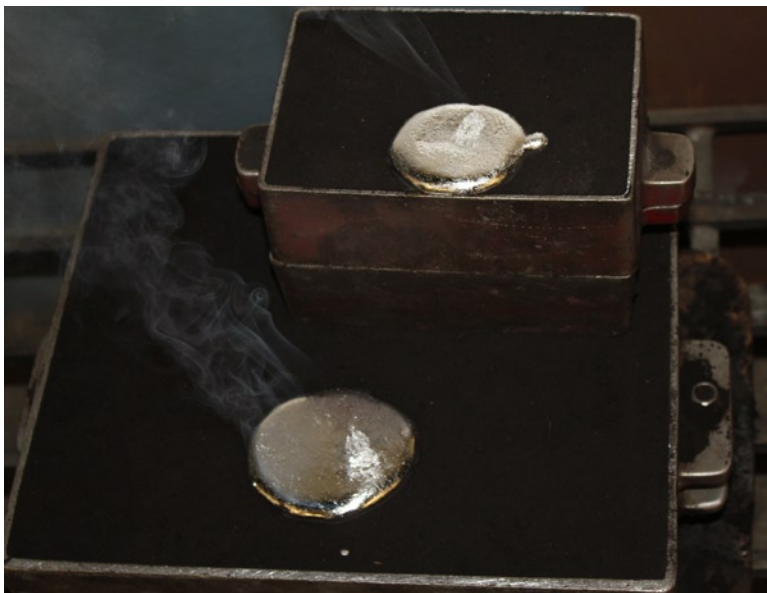
Figure 9-16. Two flasks with molten aluminum cooling
