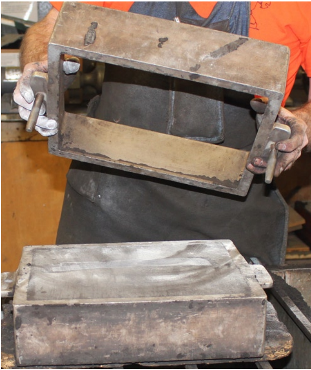
Figure 9-10. Getting ready to fill in the rest of the flask
