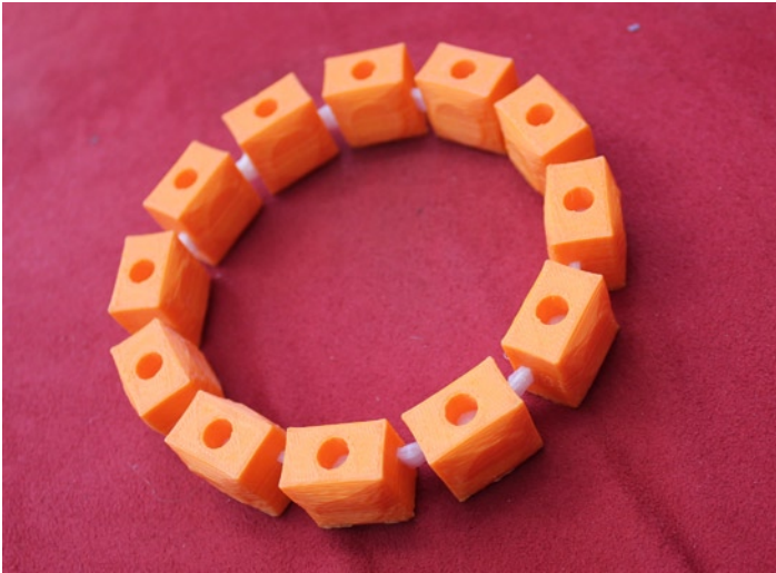
Figure 7-5. A two-material print (ABS squares and nylon connectors). Dual-material bracelet design by Diego Porqueras
