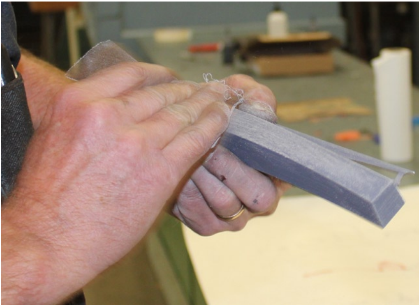
Figure 10-1. Sanding a PLA piece. (This was part of the preparation for sand casting in Chapter 9)
