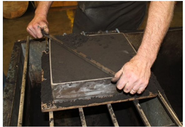
Figure 9-6. The strike-off bar gets rid of the excess sand in the flask
