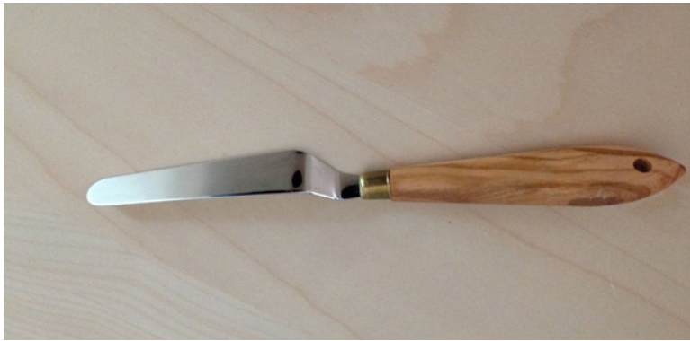
Figure 6-2. A painting knife is a good tool to remove a part from a tape-covered platform
