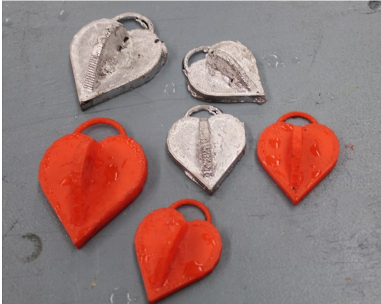
Figure 9-19. Heart patterns and finished aluminum cast pieces
