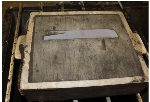
Figure 9-8. The pattern in the flask after it has been flipped upside-down
