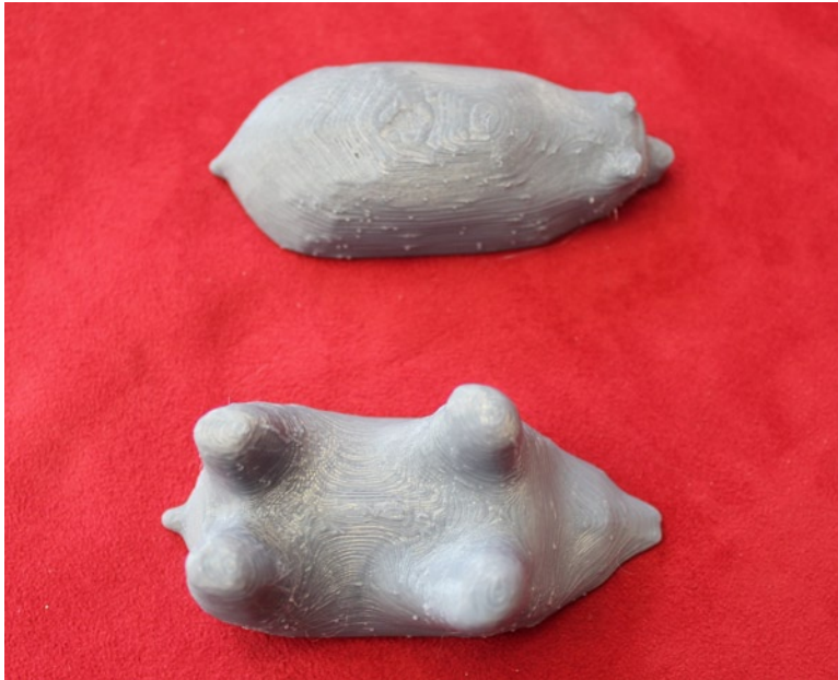
Figure 5-5. The same bear does not require support after being sliced in half, but the halves will have to be glued together
