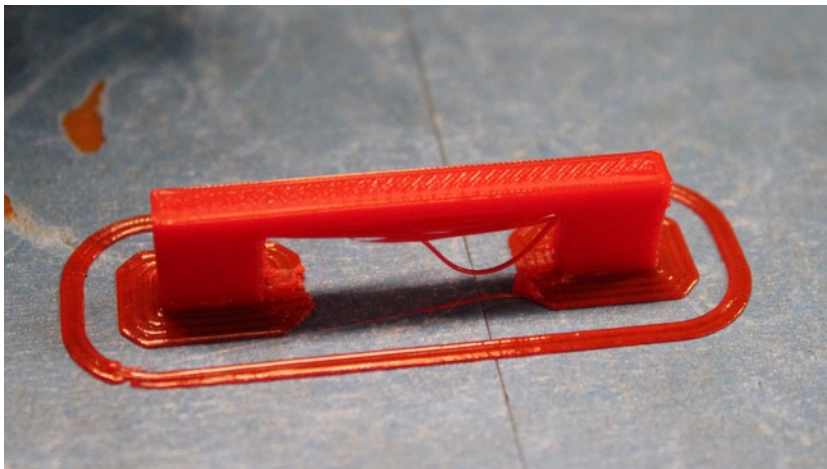
Figure 5-1. A brim and skirt (the brim is the part attached to the feet of the bridge). This print attempted to bridge a little too aggressively (see later section on bridging)
