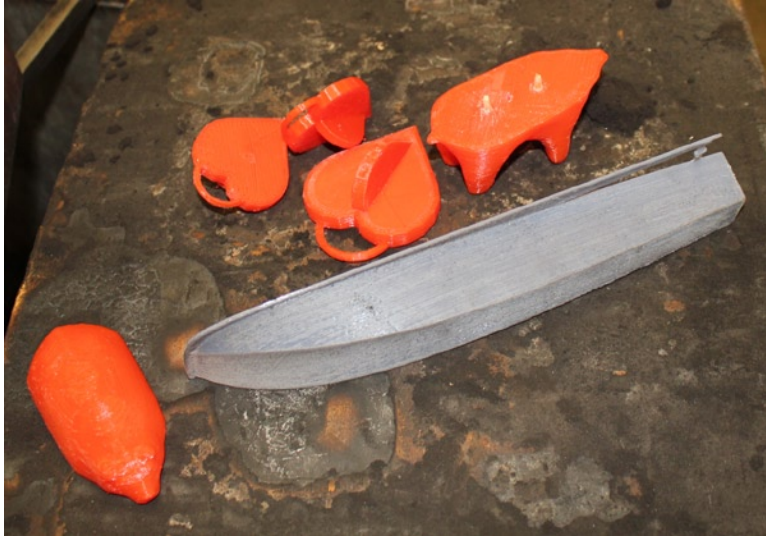
Figure 9-2. The PLA patterns used for the items in this chapter. Note the pins in the bear's lower half
