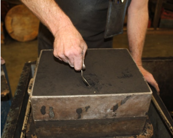
Figure 9-12. Getting the entry sprue started
