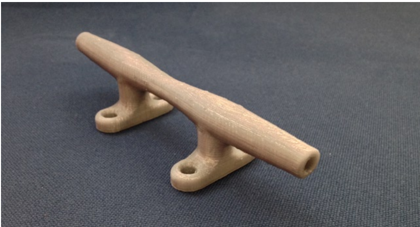
Figure 12-10. Herreshoff cleat 3D print with support removed. Created by Diego Porqueras and the Deezmaker team from original design plans, with permission from the Hart Nautical Collections of the MIT Museum. PLA print
