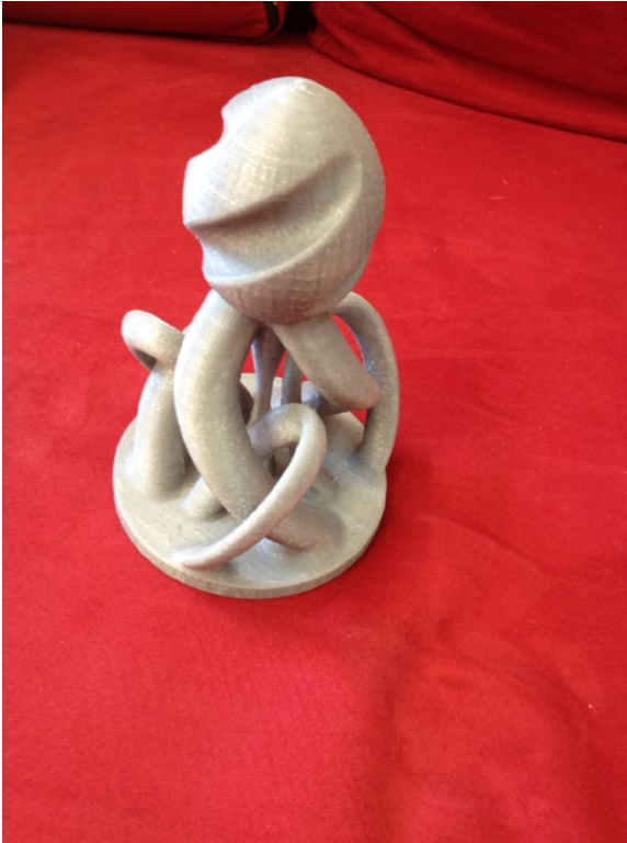
Figure 4-9. This demonstration object is 3D printable without support but would be a machinist's nightmare. Design and 3D print by Diego Porqueras
