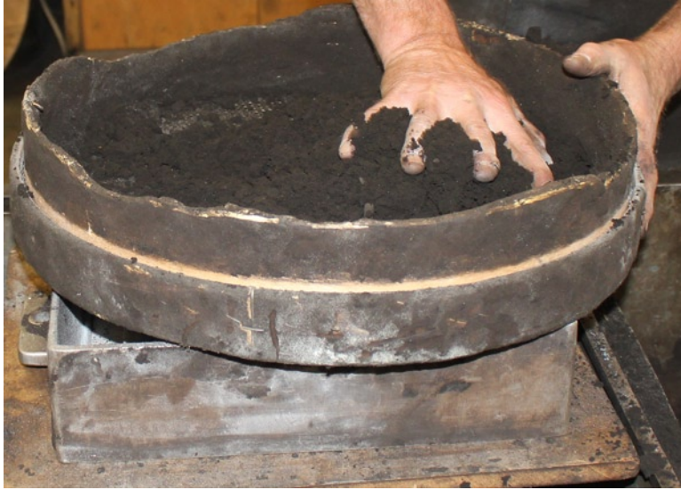
Figure 9-4. Pushing sand (mixed with oil) through the riddle into the flask
