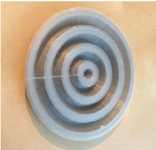
Figure 13-10. Underside of the model, with brim still on it. PLA print
