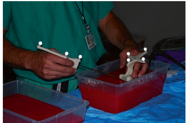
Fig. 18.9 Optical reflectors attached on plastic mounts to an ultrasound handpiece and ablation antenna. This system demonstrated superior accuracy when targeting small tumor targets in gelatin models (see Fig. 18.6)
