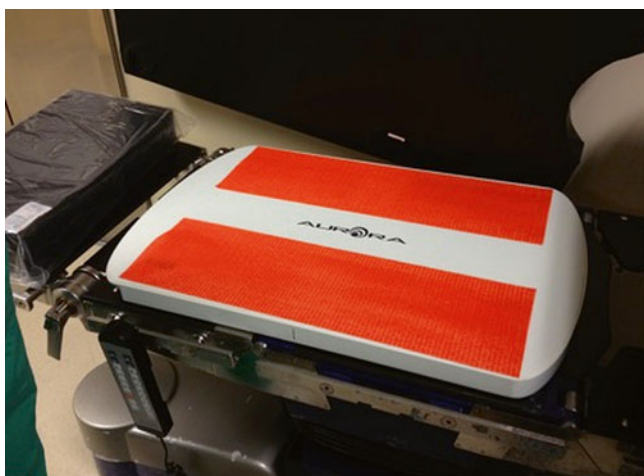
Fig. 18.15 Tabletop, flat EM field generator in position on the OR table, underneath the foam padding and patient. The device itself measures only a few cm in thickness and produces a relatively large, homogenous EM field
