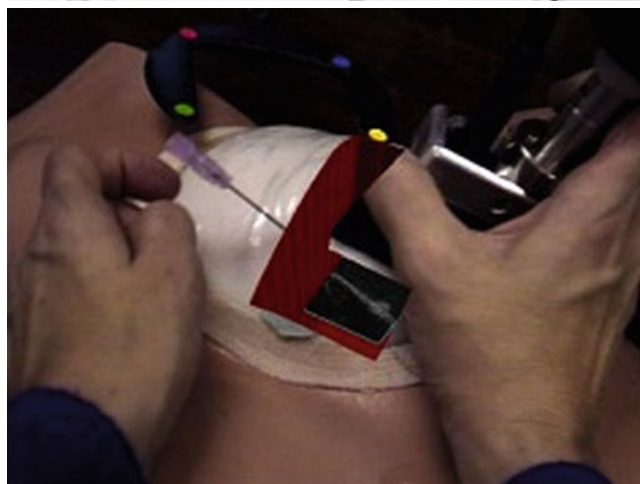
Figs. 18.3 and 18.4 Breast biopsy system (ca 1996). A mechanical arm is used to track the position and orientation of the ultrasound probe, and the live U/S scan appears inside the breast, via an augmented-reality head-worn display. Left : conceptual sketch (Courtesy of Andrei State). Right : view from the head-mounted display, showing the U/S scan on a breast phantom, with an aspiration needle (Courtesy of Andrei State)
