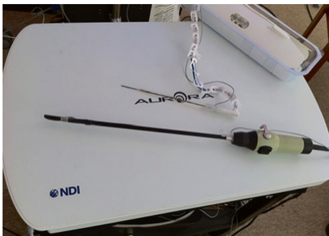
Fig. 18.14 Essential components of an electromagnetic tracking system (EMTS). A large, flat field generator, an articulating ultrasound probe, and a microwave ablation antenna
