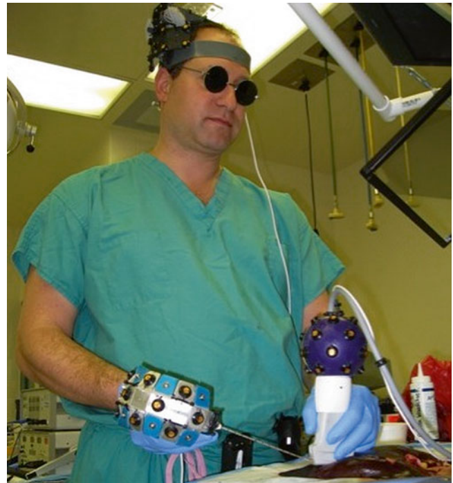
Fig. 18.5 Early guidance system prototype (ca. 2007) utilizing "active" optical sensors attached to ultrasound probes and microwave antennae and including a "head positional mount." This system was modified and refined over time
