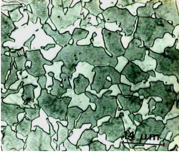
Fig. 7.49 Microstructure of dual-phase steel, an in situ composite with ferrite and martensite constituents (Rios et al. 1981). White phase is martensite, while the dark phase is ferrite
