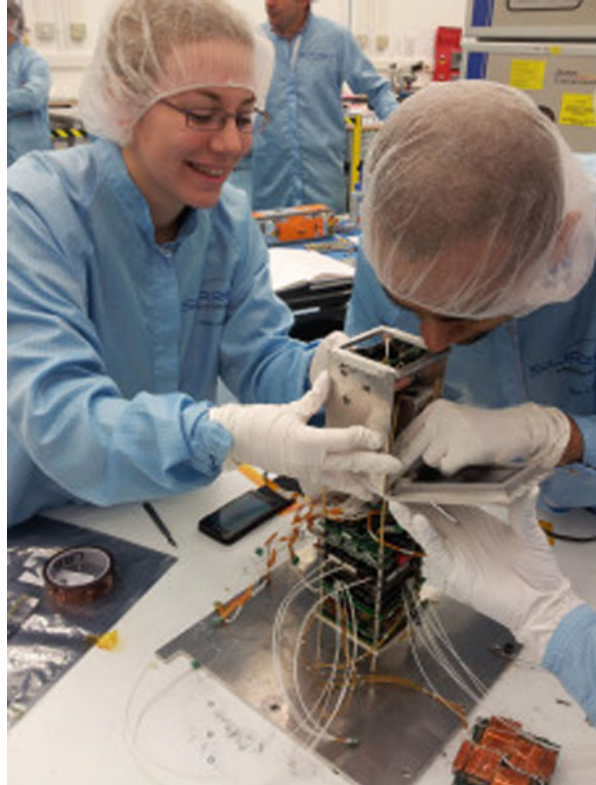
Fig. 3.7 STRaND 1 Smartphone satellite designed by Surrey Satellite Technology, Ltd
