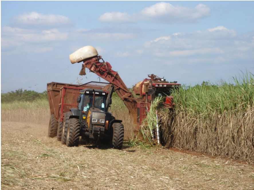
Fig. 3.12 Mechanical harvesting of green cane. (Photo courtesy of Agricef Soluções Tecnológicas Para Agricultura Ltda, Brazil; reprinted with permission)
