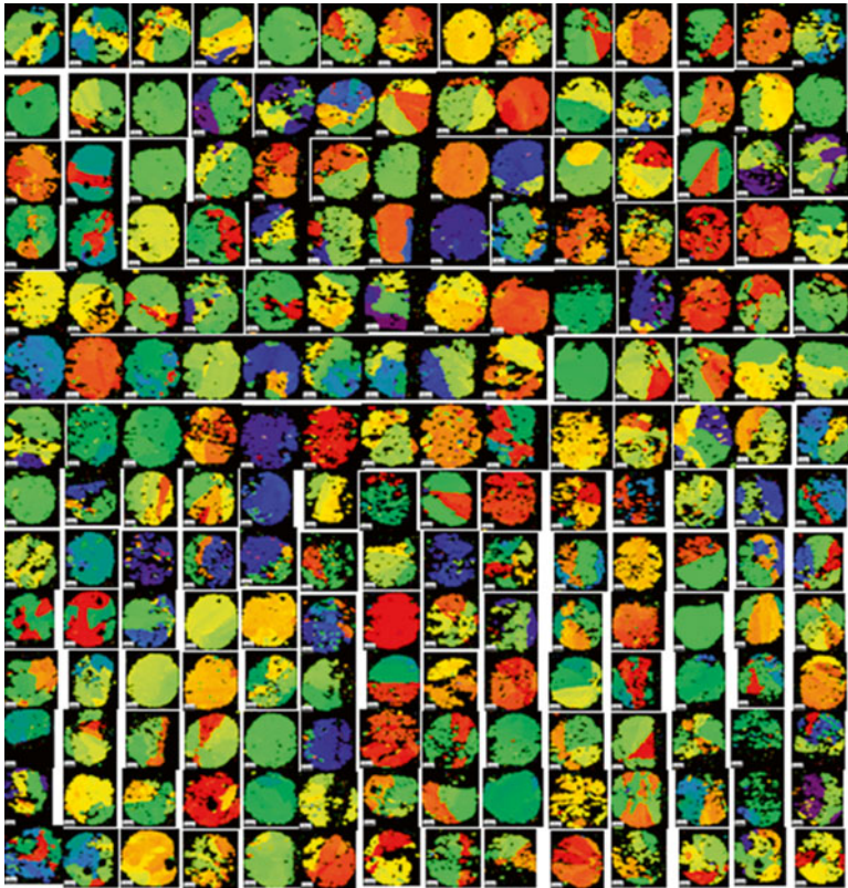
Fig. 4.7 A 14 \times 14 array of joints illustrating the variety of orientations of single and tri-crystal orientations. The color code is based upon the c -axis orientation with respect to the substrate. Ball D13 (4th row, 13th column) is examined in detail in Fig. 4.5
