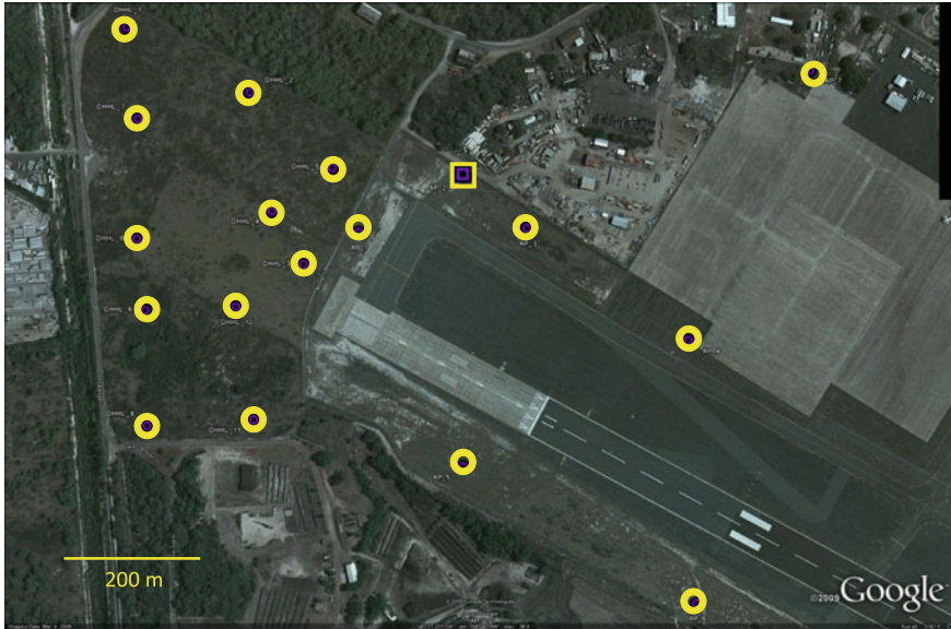
Fig. 6 Pyranometer array at the Kalealoa Airport in southwestern Oahu (Hawaii, USA). Circles represent locations of 1 s GHI sensors, and the square represents the location of the RSR 3 s sensor. Although the distance between stations is variable, the east-west extent of the array is approximately 900 m, and the north-south extent is approximately 800 m, and the shortest distance between two stations is \sim 100 m
