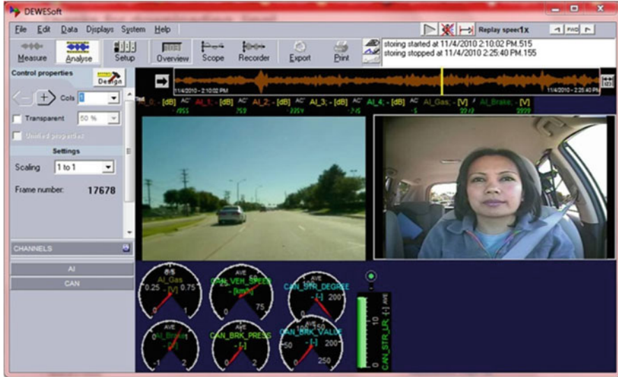
Fig. 11.2 Dewesoft software used for recording and exporting the data. The figure shows the frontal and road videos. It also shows the instantaneous values of various CAN-bus signals
