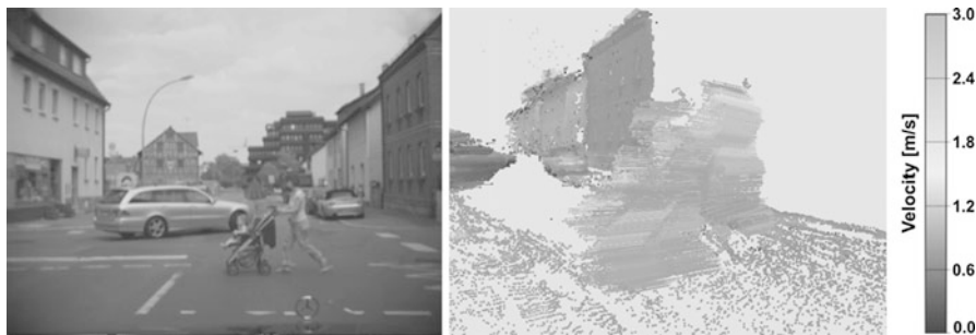
Fig. 2.2 Left : Typical traffic scene. Right : Motion field, estimated by the Dense6D algorithm proposed in this chapter. The color encodes the velocity of the observed points
