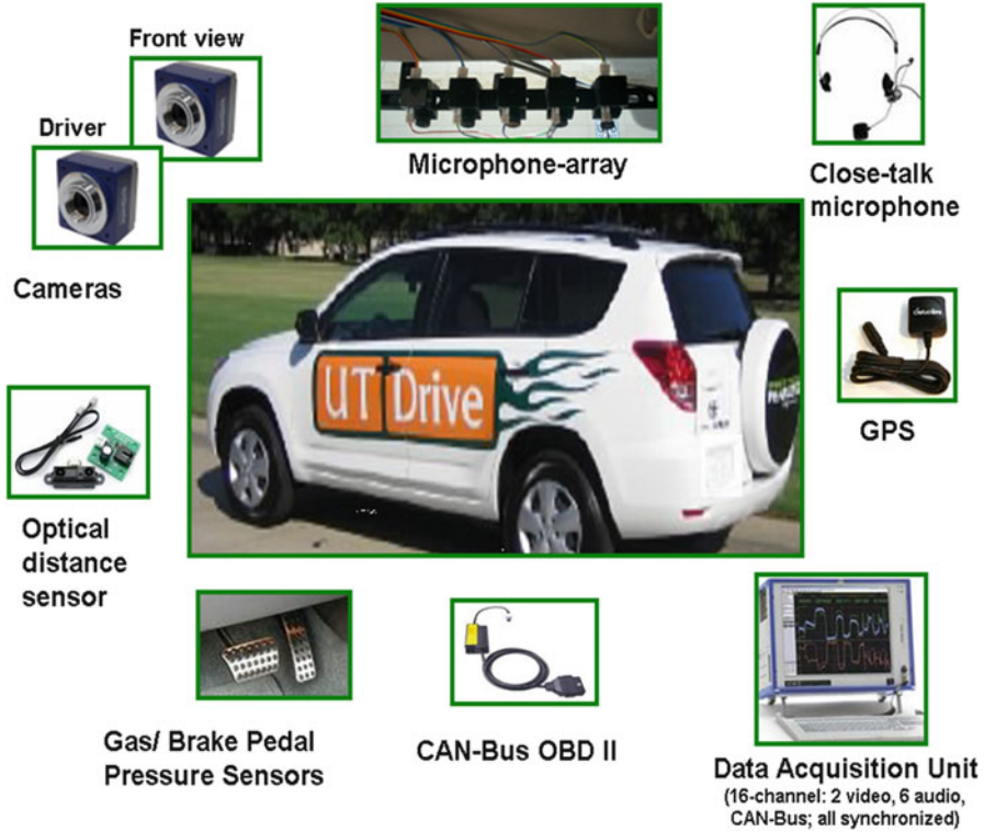
Fig. 10.2 Instrumented UTDrive data collection vehicle along with the sensors [10]
