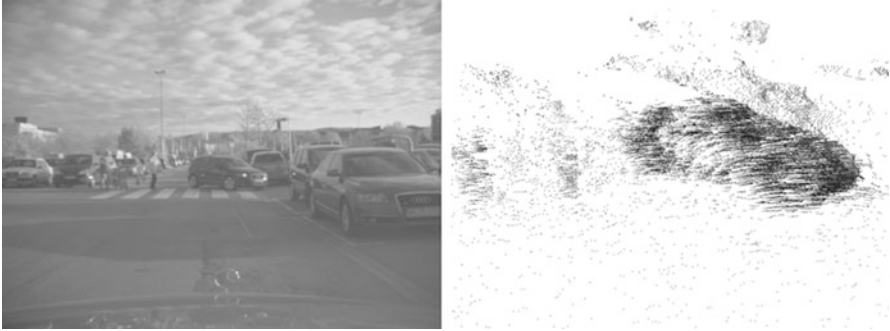
Fig. 2.8 Left: Typical traffic scene. Right: Corresponding 3D motion field, estimated by the Dense6D algorithm proposed in this chapter
