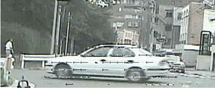
Fig. 15.9 Vehicle crossing the intersection at a traffic light stop. Superimposed motion vectors present a relatively high intensity in the direction of apparent motion when they are located in the car area while they are nearly zero in the rest of the image
