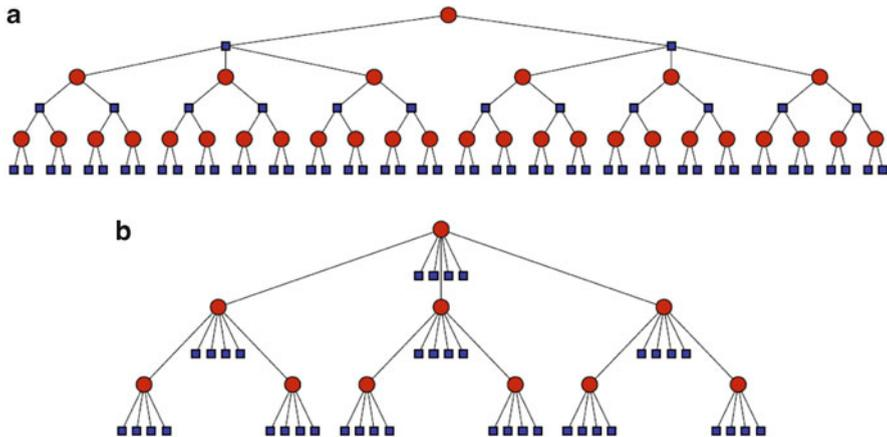
**Fig. 8.1** Examples of traditional and multi-horizon scenario trees. (a) Traditional scenario tree structure with a combination of strategic and operational uncertainty. (b) Multi-horizon tree with the same number of strategic branchings but double number of operational branchings as the traditional tree
