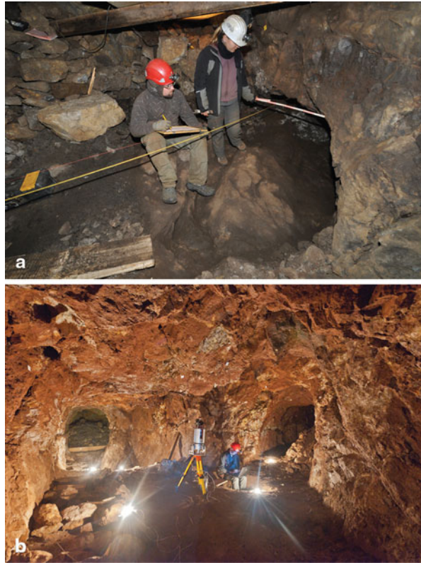
Fig. 7.12 a Traditional mapping underground, Slovakia, Poniky. Medieval to modern times mine. b Laser scanning underground, Sakdrissi Gold Mine. (a DBM, Th. Stöllner; b DBM, Th. Rabsilber)
