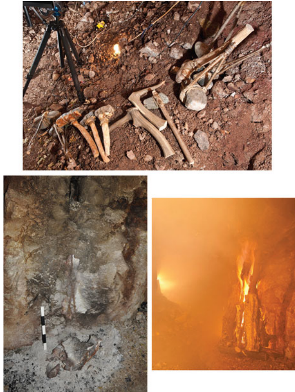
Fig. 7.14 Sakdrissi, Georgia—hammerstone kit as prepared by B. Craddock in 2011 used for the fire-set experiment 3/2011 underground ( top ). Exfoliation of wall parts after the fire-set ( bottom left ) and the heavy smoke during the experiment ( bottom right ). (Photos: DBM, K. Stange)
