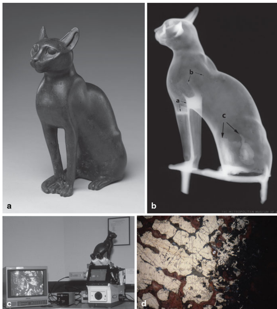
Fig. 12.10 a Cat sarcophagus, Egyptian, Macedonian-Ptolemaic Period (332–30 B.C.). Hollow cast bronze. H. with tangs 32.0 cm. New York, The Metropolitan Museum of Art, Harris Brisbane Dick Fund, 1956 (56.16.1). b X-ray radiograph of bronze cat sarcophagus; the hollow body, head, and legs appear more radiotransparent than the solid ears, paws, tail, and tangs. Radiopaque bands along the top of the legs ( a ) indicate where wax, now reproduced in cast metal, was used to join separate cores. Small rectangular radiotransparent spots indicate original locations of now-rusted iron core supports ( b ) Two cast-in repairs are proportionately more radiopaque than the surrounding walls. ( c ) Sarcophagus placed directly over microscope objective to avoid sampling during metallurgical examination. d Polished section viewed under conventional light showing dendritic structure; superficial and intergranular cuprite corrosion appears red. The latter, when present, is considered a highly reliable indicator of an extended period of burial. (Images © The Metropolitan Museum of Art)
