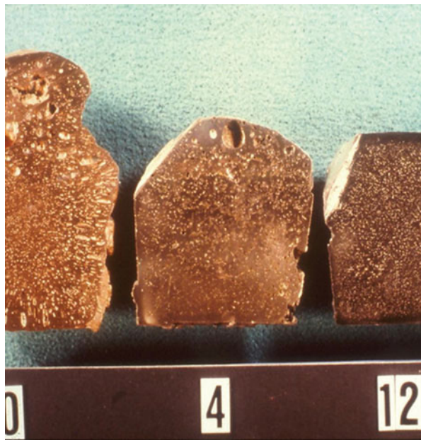
Fig. 8.22 Sections of the arsenical copper containing 0, 4 and 12 % As, showing an inverse relationship between arsenic content and porosity. (Author's (BSO) photograph)
