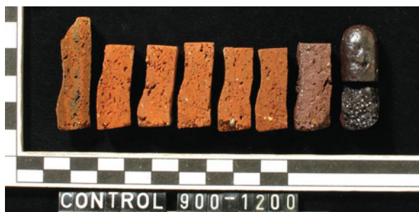
Fig. 6.21 A sequence of samples employed for refrining experiments to assess the refractoriness of Qantir crucibles. (Photo: Axel Krause / Excavation Qantir)
