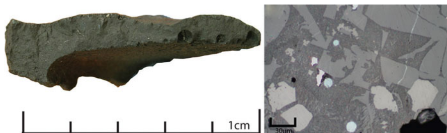
Fig. 26.5 a Section of slag sample (117). b Photomicrograph of polished section showing iron silicate phases and sulfide inclusions. (Photos courtesy of R. Doonan)
