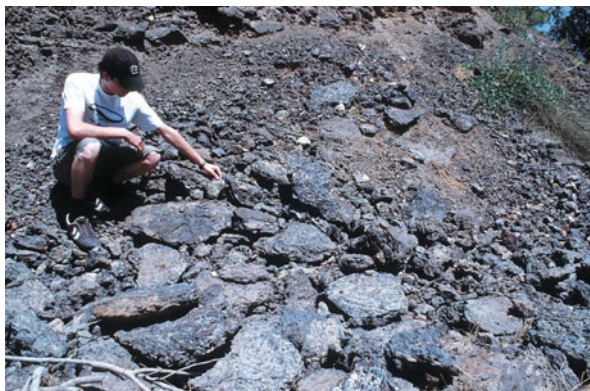
Fig. 5.2 Huge slag heaps accumulated close to the copper deposit of Skouriotissa, Cyprus, during the Roman and Byzantine Period. Tap slags with a weight of 50 kg or more were produced by smelting copper ores. Note the flow structures of the slag cakes, which is very similar to the frozen texture of volcanic rocks. They indicate that these slag cakes were tapped from a smelting furnace in the fully liquid state and solidified outside the furnace very quickly
