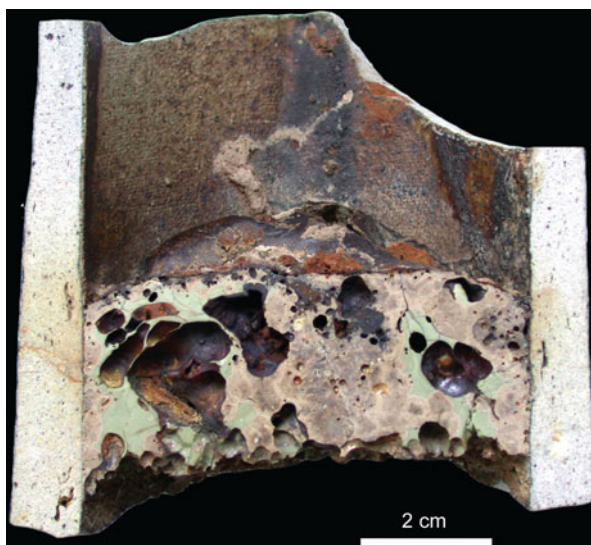
Fig. 6.7 Section through part of a medieval steel-making crucible from Akhsiket, Uzbekistan. Note the clean interface and lack of interaction between the slag and the white ceramic, denoting the high refractoriness of the latter. (Photo: Marcos Martín-Torres)
