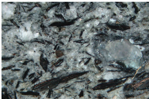
Fig. 6.20 Photomicrograph of a polished cross section of a post-medieval crucible, showing abundant flakes of black graphite. Image width is ca. 2 mm. (Photo: Marcos Martínón-Torres)
