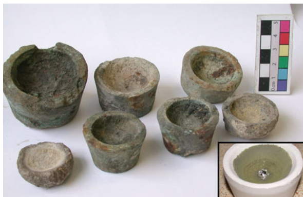
Fig. 6.17 Some archaeological cupels from the site of Kapfenberg, Austria, made with a mixture of bone ash and wood ash, now heavily impregnated with lead and other base metal oxides. Inset: a modern cupel with the silver regulus still in place. (Photos: Marcos Martín-Torres)
