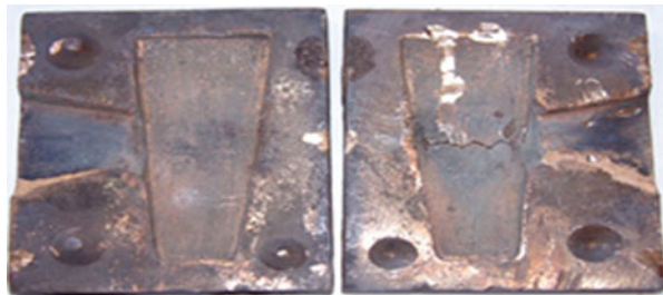
Fig. 8.27 Bronze moulds used in casting experiments started to crack after the ninth casting. (Wang and Ottaway 2004, Figs. 5 and 13)
