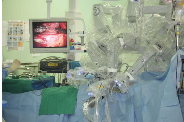
Fig. 13.8 Docking of robotic surgical system. A face-down 30° endoscope is used for visualization of the surgical field. A 5 mm Maryland forceps and 5 mm Harmonic curved shears are equipped on either side of the endoscope
