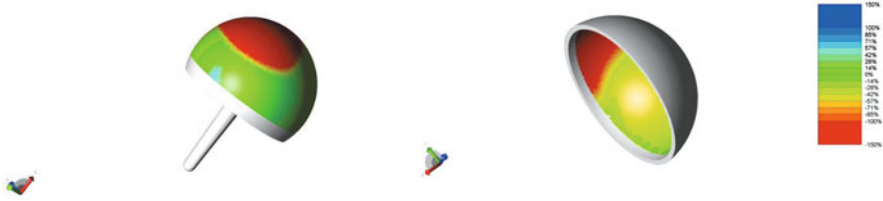
Fig. 5.1 Typical wear map of a failed hip resurfacing. Red areas indicate wear of greater than 10 \mu\text{m} . Volumetric wear rate was greater than 30 \text{ mm}^3/\text{year} in this case. Typically as is seen in cases of excessive bearing surface wear, blood Co concentration was 92 \mu\text{g/L} and Cr was 40 \mu\text{g/L} . Joint fluid levels showed the usual paradoxical concentration ratio associated with excessive bearing wear with Cr concentration of 11,000 \mu\text{g/L} and Co 4,500 \mu\text{g/L} . Gross metallosis and osteolysis was encountered at revision surgery though soft tissue necrosis was not extensive. Note that even with such elevated wear rates a large proportion of the bearing surface remains within the as-manufactured form ( green areas )
