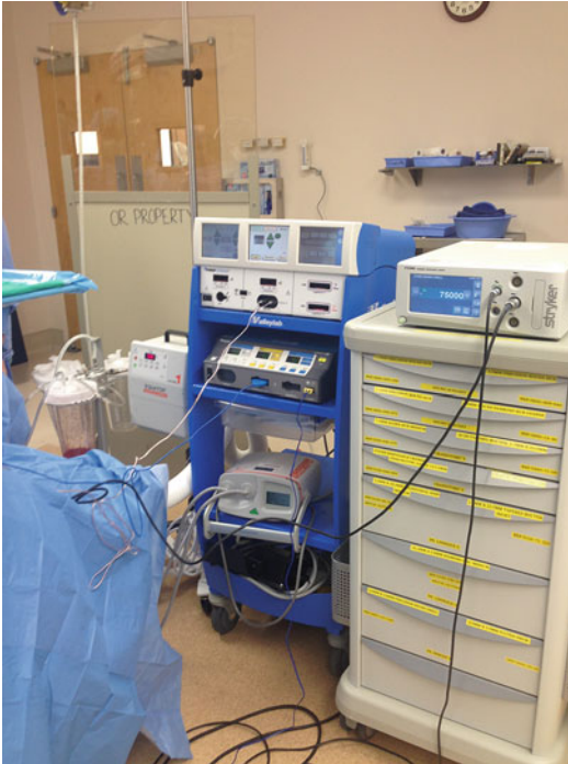
Fig. 1.5 The electro-surgical units are shown in the top and middle of the blue cart
