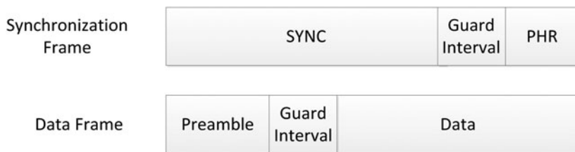
Fig. 9 Frame structure for transmit-only MAC protocol for wireless body area network (WBAN)
