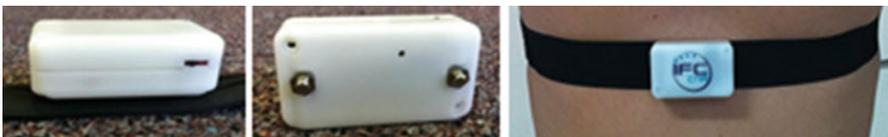
**Fig. 10.7** The customized ECG sensor
