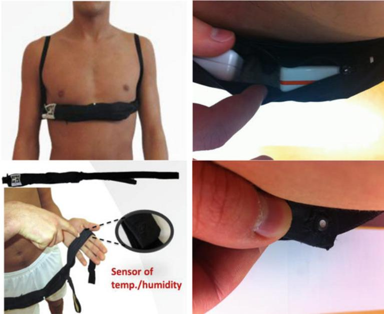
**Fig. 10.15** The chest strap encapsulating the sensor modules
