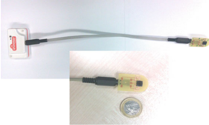
Fig. 10.12 Prototype of the temp sweat index sensor connected to the Shimmer acceleration module
