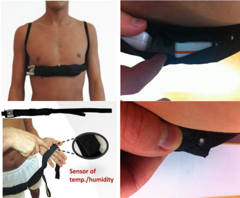
Fig. 10.15 The chest strap encapsulating the sensor modules
