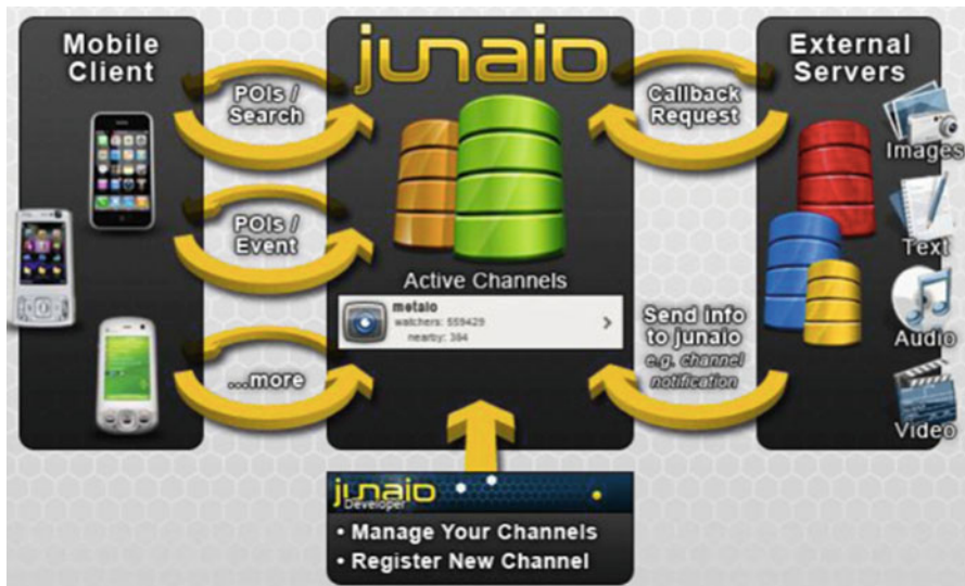
Fig. 2 The Junaio client/server architecture
