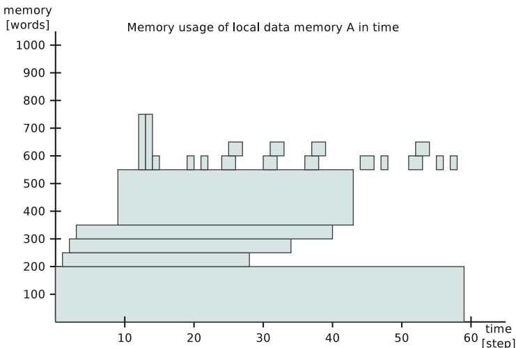
Fig. 9.5 Mapping of variables to local memory A
