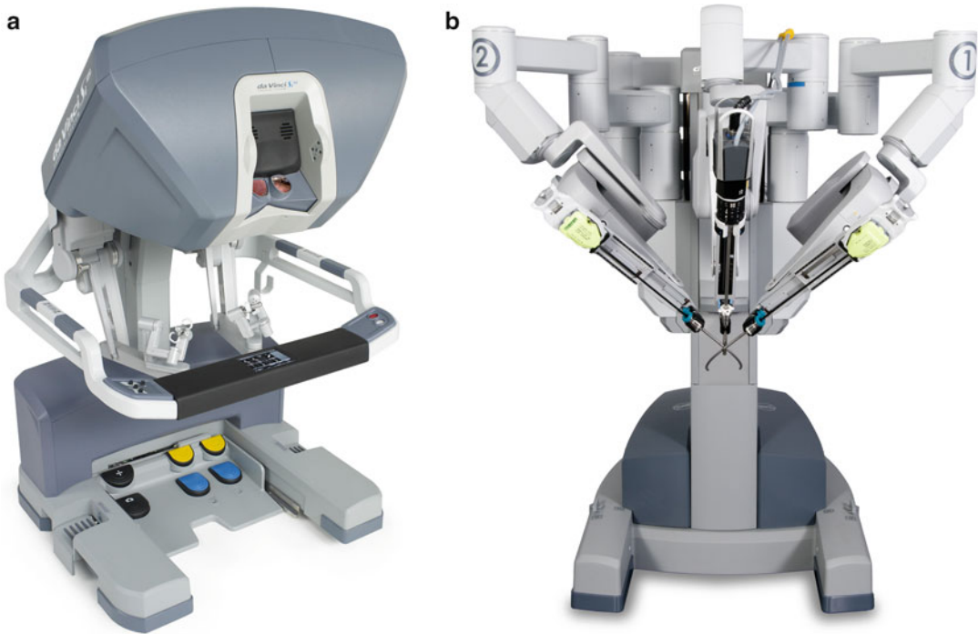
Fig. 38.1 (a and b) The da Vinci Si HD surgical system: surgeon console and patient cart (© 2009 Intuitive Surgical, Inc., with permission)
