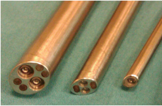
Fig. 29.4 A comparison between the original robotic scopes for the Standard da Vinci camera. ( left , 12 mm 3D; middle , 8.5 mm 3D; right , 5 mm 2D). The 5 mm 2D scope is no longer manufactured
