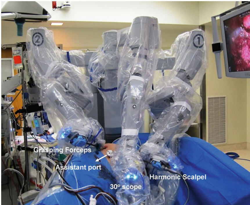
Fig. 25.3 Intraoperative image depicting the position of the robotic system in a robotic right LT adrenalectomy
