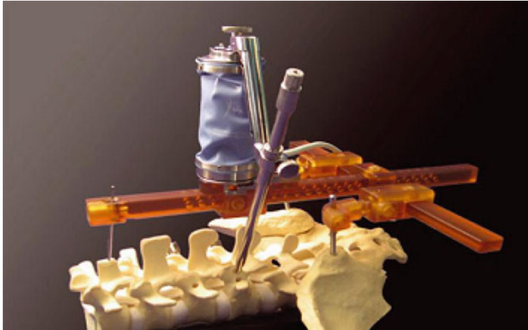
Fig. 38.8 The SpineAssist (Mazor Robotics Ltd, Israel) (From Stürer C, Ringel F, Stoffel M, Reinke A, Behr M, Meyer B. Robotic technology in spine surgery: current
