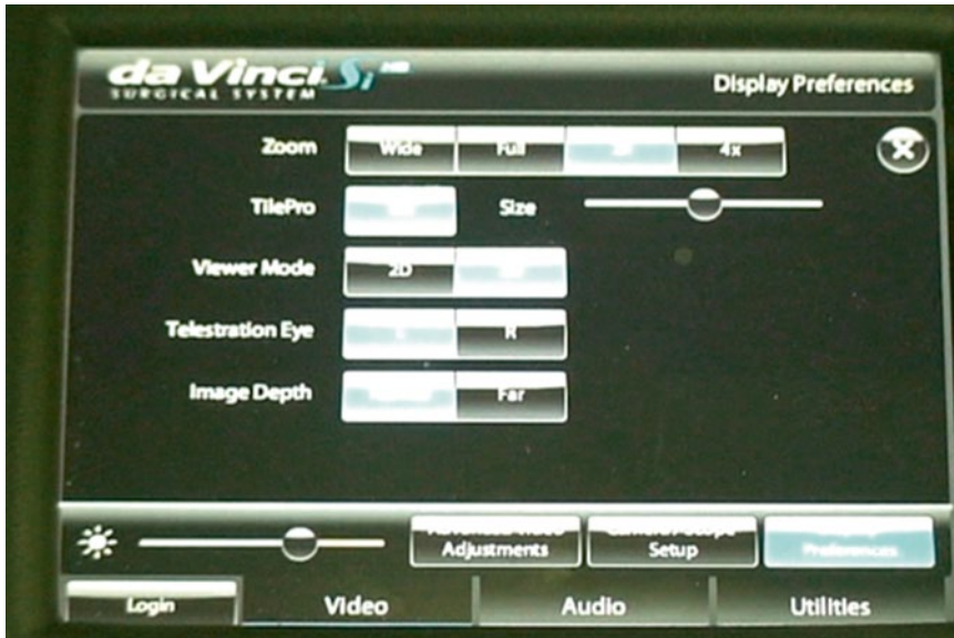
Fig. 35.2 TilePro can be activated by using the touch pad panel at the surgeon console. The surgeon can control the video input on and off by tapping the foot pedal for the camera
