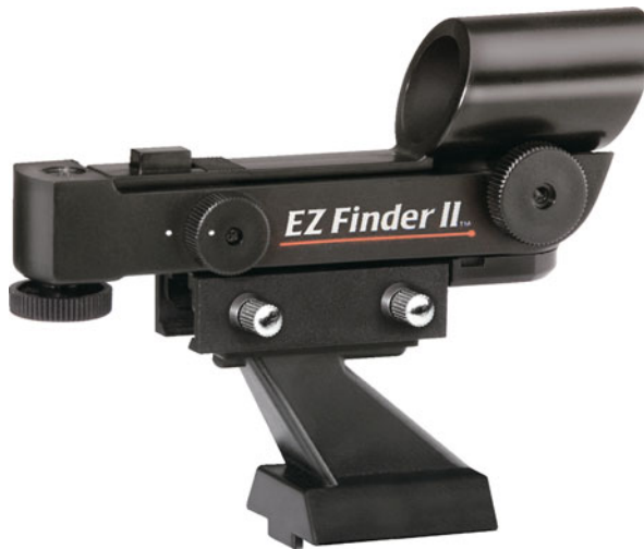
Fig. 7.4 A unit-power (non-magnifying), reflex-sight finder like that now widely used on telescopes in place of (or in conjunction with) conventional optical finders. It works simply by superimposing a tiny LED red dot focused at infinity on a 10^\circ view of the sky, showing exactly where the telescope is pointed. Courtesy of Orion Telescopes & Binoculars
