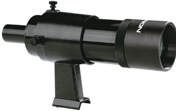
Fig. 7.3 A conventional straight-through optical finder. Unlike this 9×50, finders on many small telescopes are greatly undersized and often are all but useless. Ideally, a finder should be one quarter of the aperture of the telescope it’s riding. But Go-To technology has made this less of an issue today for scopes so equipped. Courtesy of Orion Telescopes & Binoculars
